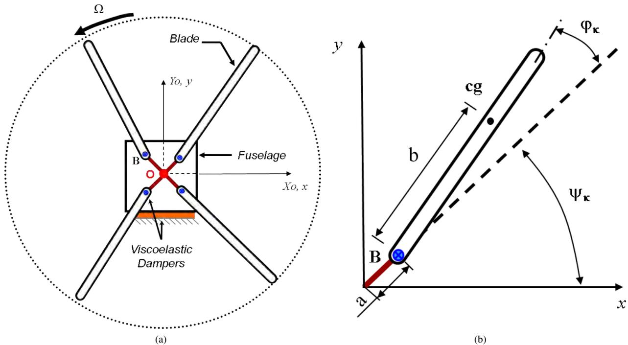
Figure 1: Sketch of the Mechanical System: (a) General View and (b) Blade View
