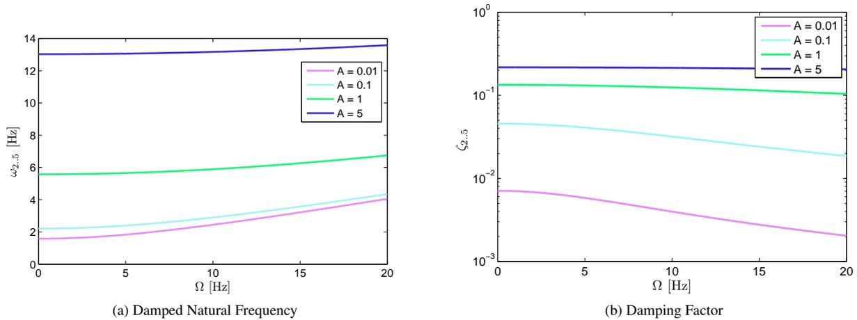
Figure 7: Parametric Analysis on the Evolution of the Dynamical Properties of the Blades for Different Viscoelastic Dampers: (a) Damped Natural Frequency and (b) Damping Factor
