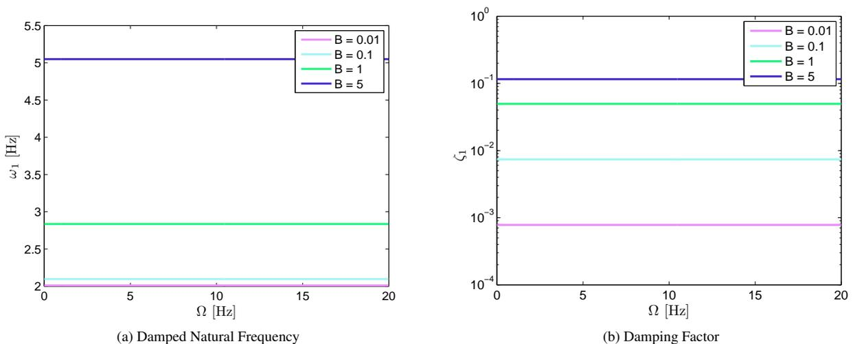
Figure 6: Parametric Analysis on the Evolution of the Dynamical Properties of the Fuselage for Different Elastomeric Dampers: (a) Damped Natural Frequency and (b) Damping Factor
