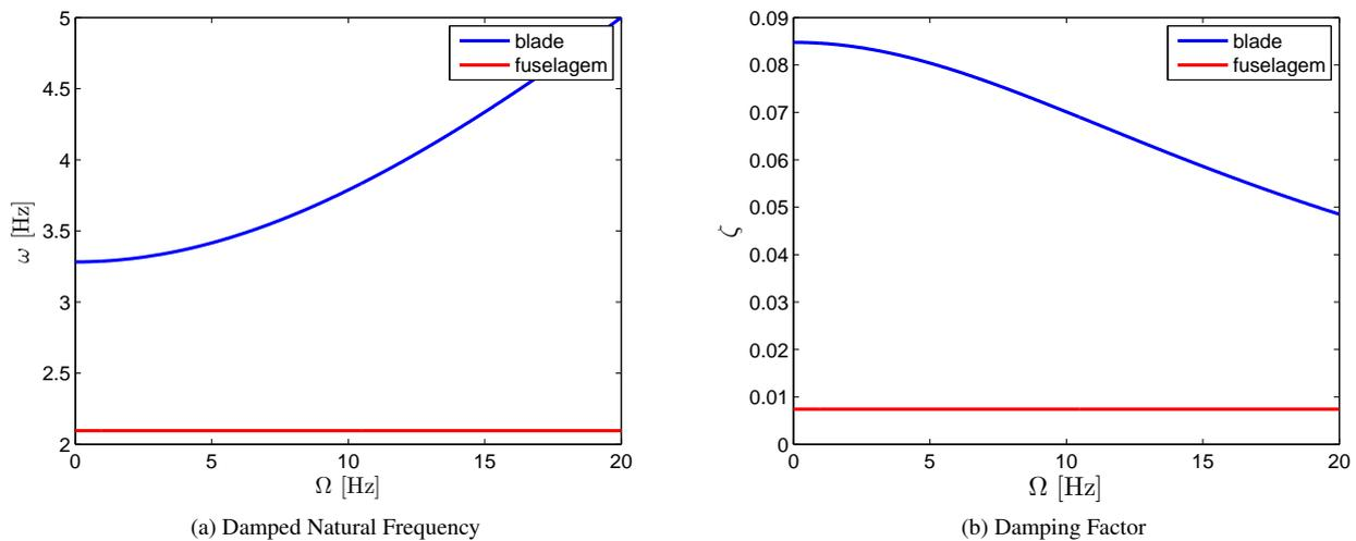
Figure 4: Evolution Dynamical Properties of the Fuselage and Blades with Viscoelastic Dampers: (a) Damped Natural Frequency and (b) Damping Factor
