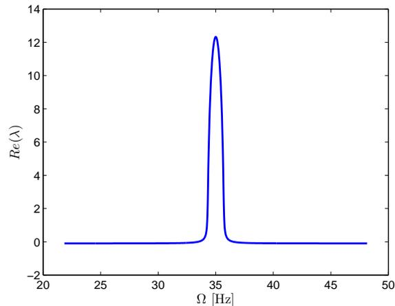
Figure 5: Stability of the Helicopter at Parametric Resonance of First Order -  $\Omega = \omega_1 + \omega_n$ ,  $n = 2..5$
