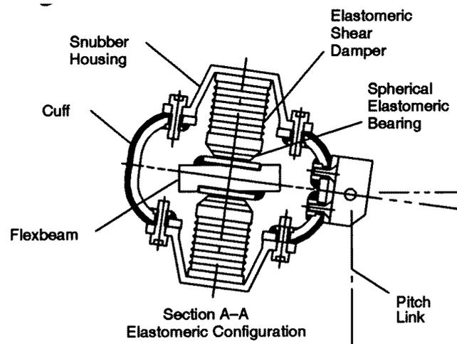
Figure 2: Schema of an Elastomeric Rotor Configuration (obtained from Panda *et al.* (1996))
