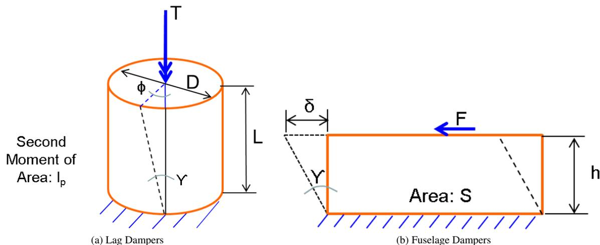
Figure 3: Geometrical Characteristics and Deformations (dashed lines) of the Viscoelastic Material at: (a) Lag Dampers and (b) Fuselage Dampers
