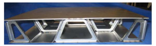
Figure 2. Thermally Integrated Structural Sandwich Core (TISSC) - NASA concept.
