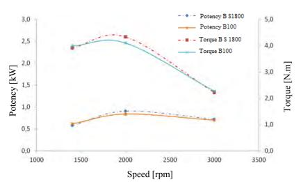
Figure 4. Engine performance at full load diesel use (S1800 B) and soybean ethyl ester (B100) (Petter AA1 Performance Motor Full Load)
