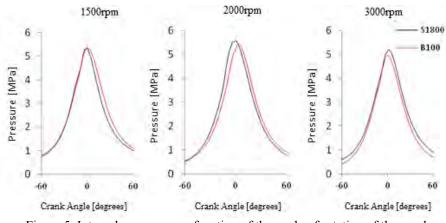
Figure 5. Internal pressure as a function of the angle of rotation of the crank.
