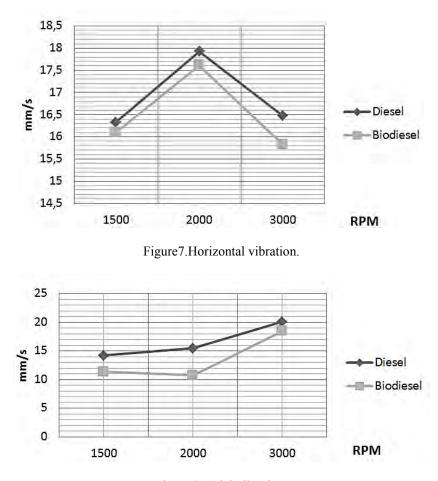
Figure 8.Axial vibration.
