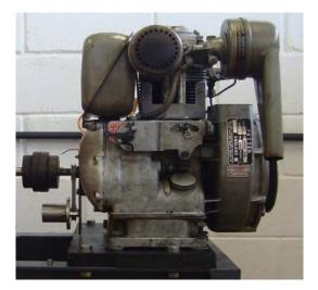
Figure 1. Engine, model Petter AA1, single-cylinder, naturally aspirated air-cooled.
