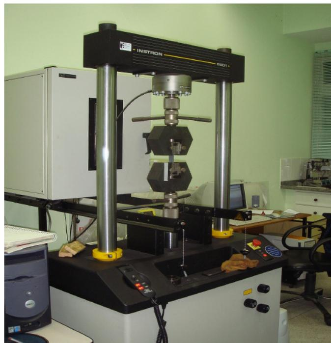
Figure 7 – Testing machine INSTRON 8801.
