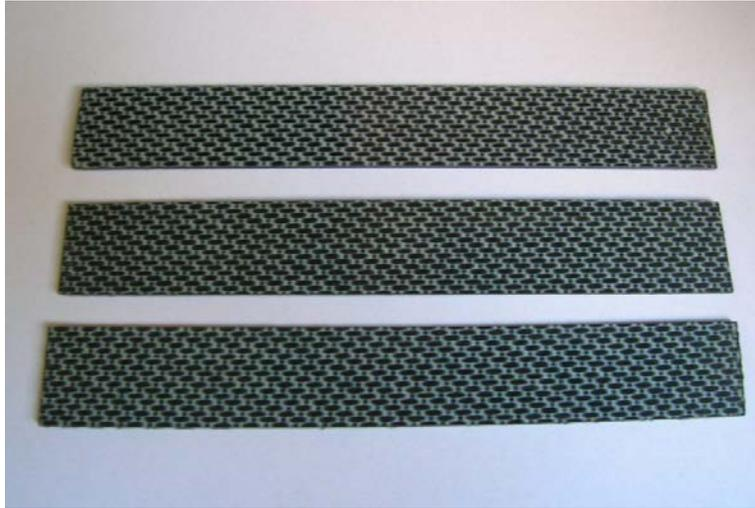
Figure 8 – Specimens used in the tensile tests.
