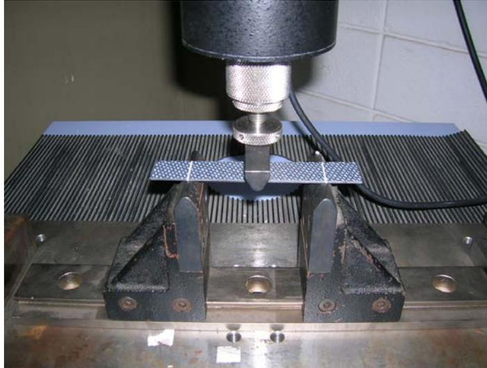
Figure 4 – Positioning of the specimen in testing machine.
