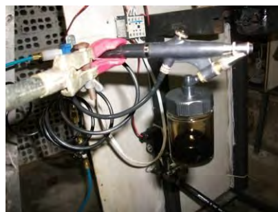
Figure 4. Compressed air/BO25 injector nozzle
