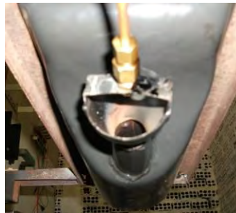
Figure 3. LPG injector nozzle
