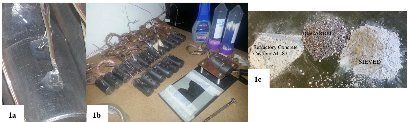
Figure 1. 1a) Fixing equidistant thermocouples. 1b) Capacitive-welding materials used. 1c) Refractory concrete sifted.
