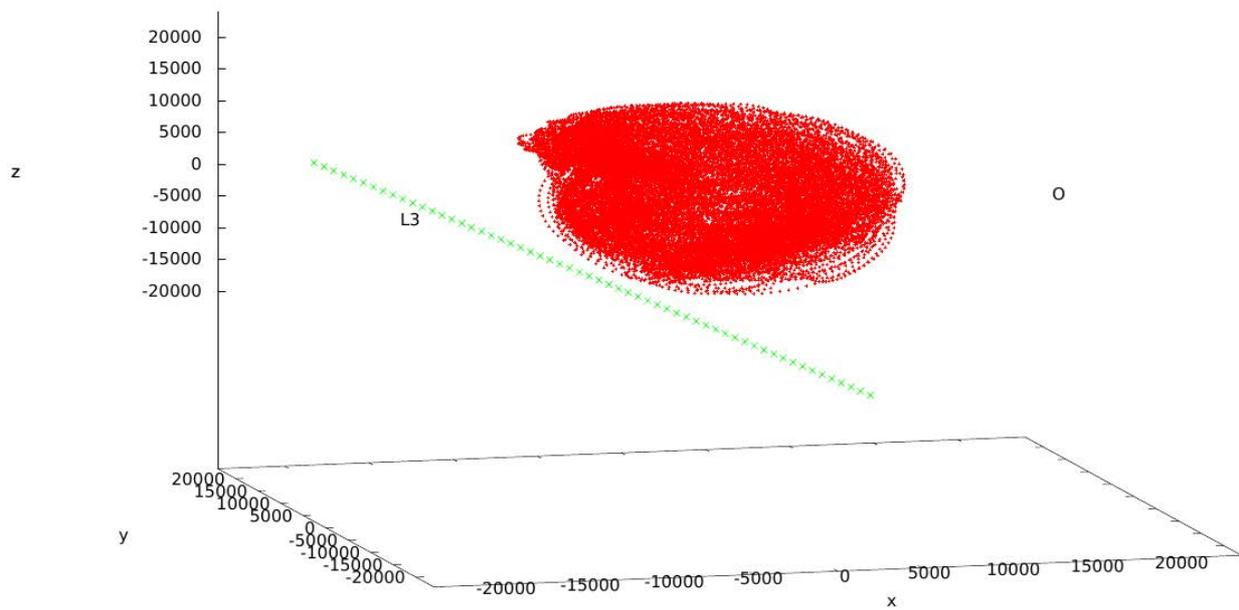
Figure 3. A set of trajectories corresponding to some of the largest quasi-periodic orbits for different values of orbital inclination (several quasi-periodic orbits for each inclination) and the trajectory of the New Horizon spacecraft (straight line in green). The open circle on the right indicates the position of Charon.
