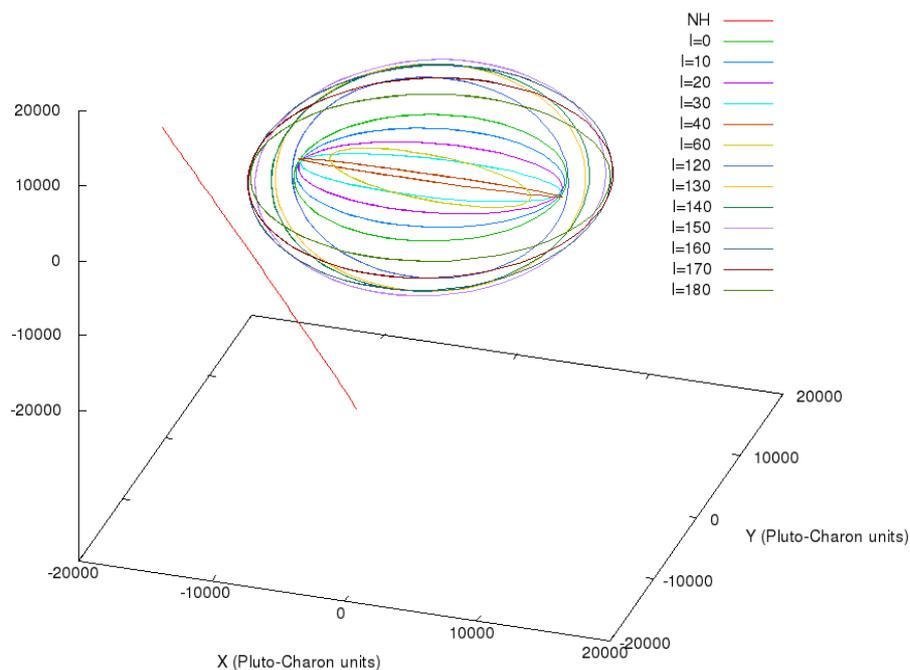
Figure 2. A set of trajectories corresponding to periodic orbits for different values of orbital inclination (one periodic orbit for each inclination) and the trajectory of the New Horizon spacecraft (straight line in red).
