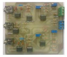
Figure2. Board of analog hardware for eletromyographic signal conditioning
