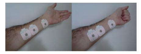
Figure 7. Surface Electrodes Arrangement
