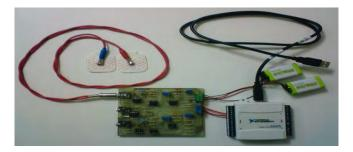
Figure 4 - System for electromyographic signal acquisition
