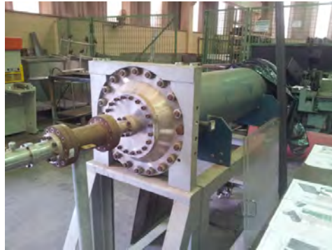
Figure 6. Vitiated Air Generator's overview.
