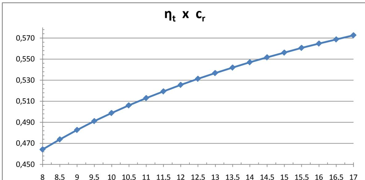
Figure 12. Thermal efficiency ( $\eta_t$ ) versus the compression ratio ( $c_r$ ) for  $k = 1,3$ .
