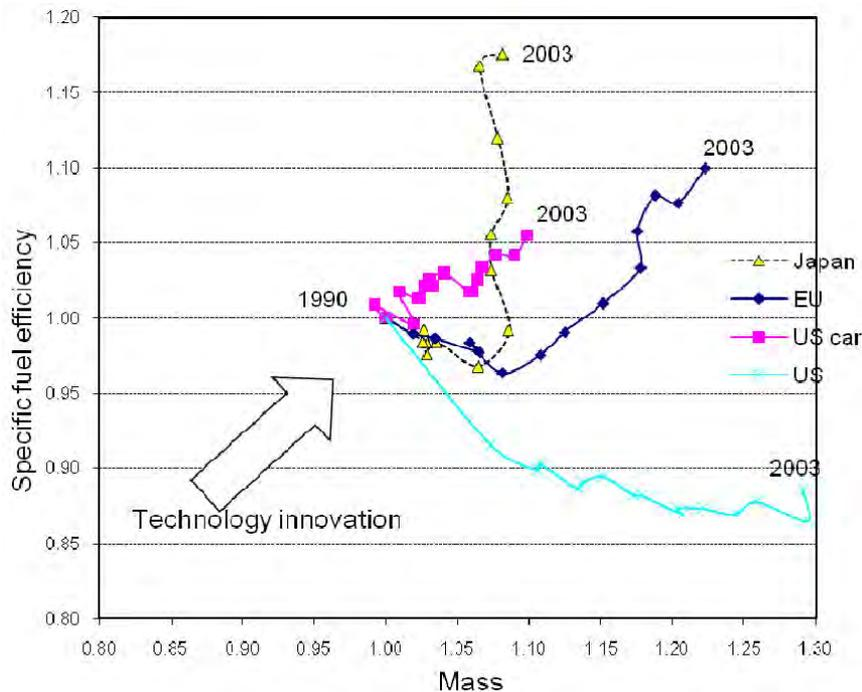
Figure 6. Fuel efficiency and mass trends (1990 = 1). Source: Onoda (2008).
