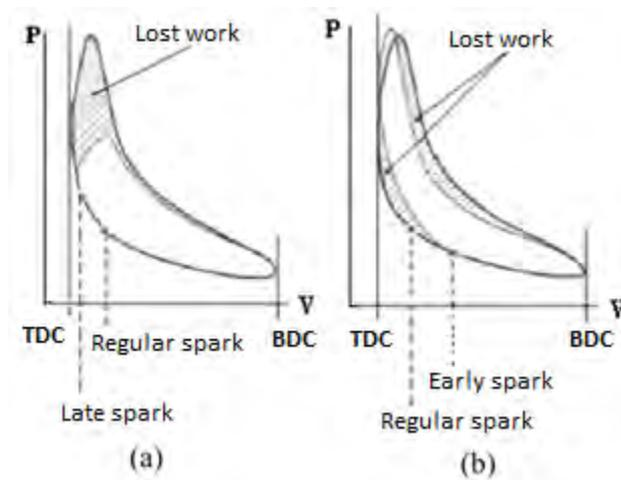
Figure 11. Influence of the ignition timing in the real Otto Cycle, (a) late spark, (b) early spark. Source: Giacosa (1988) apud Malfatti (2009).
