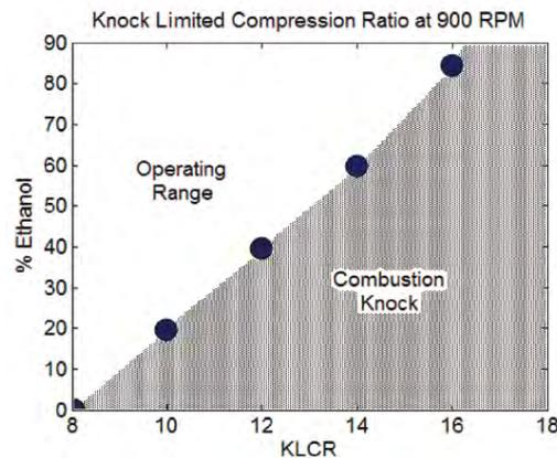
Figure 10. Experiment of a variable compression ratio engine and a variable blend of gasoline and ethanol. Source: Cooney et al (2009).
