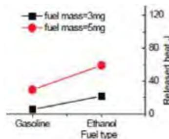
Figure 9. Comparison of fuels burn (NVO period) in stoichiometric mixtures. Source: Yang et al (2010).
