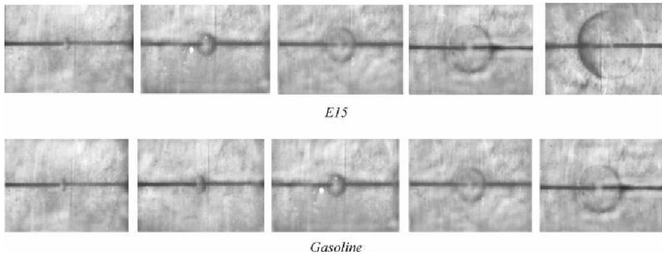
Figure 8. Flame core growth captured by schlieren camera for stoichiometric mixtures of E15 and Gasoline. Source: Liao et al (2005).
