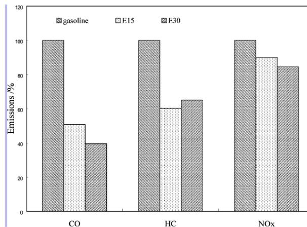
Figure 7. Emissions variations related to ethanol blend in gasoline (E15 and E30). Source: Liao et al (2005).
