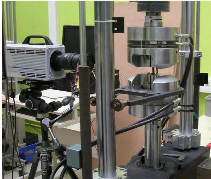
Figure 2. The mounting apparatus of DIC technique
