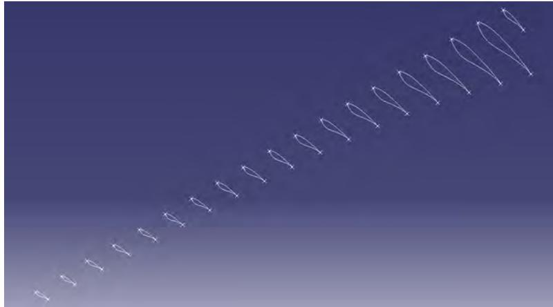
Figure 3. Airfoils along the Blade
