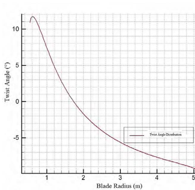
Figure 1. Twist Angle Distribution
