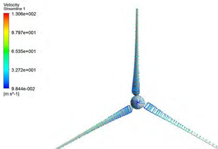
Figure 11. Streamlines on the Surface (Suction Side)
