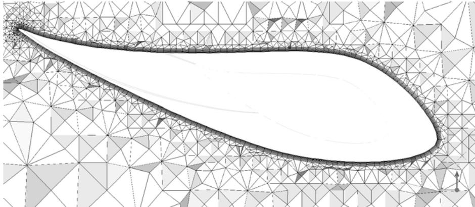
Figure 6. Hybrid Mesh with Prismatic Elements
