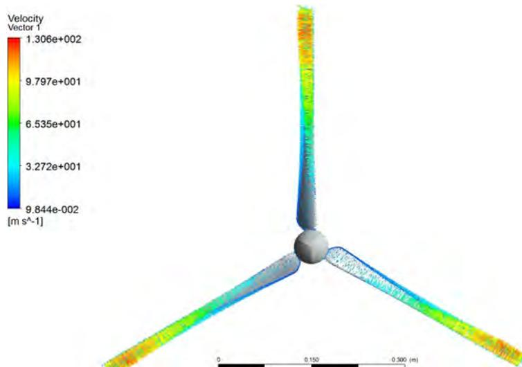
Figure 10. Relative Velocity Vectors
