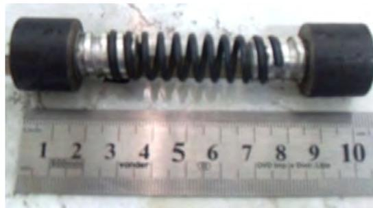
Figure 7. SMA helical spring.
