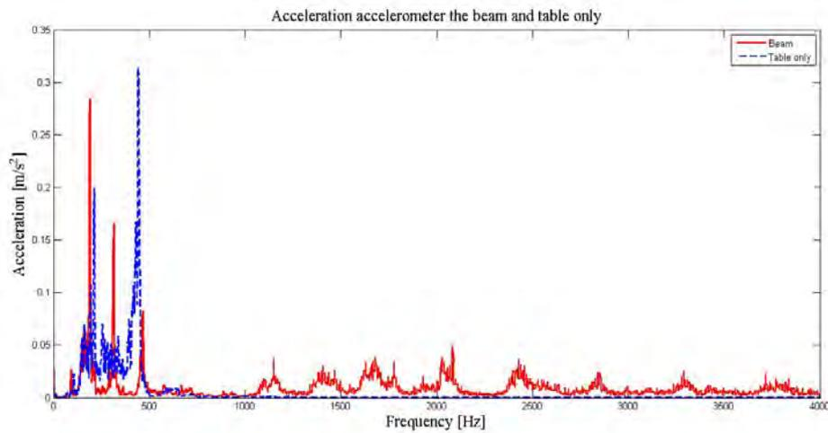
Figure 3. Frequency response of the support only (in blue) in terms of acceleration induced by noise white.
