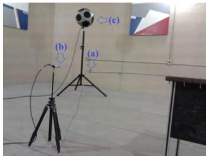
Figure 1. Beam with acelerometer (a), microphone (b) and omnidirectional sound source (c) in the reverberant room.
