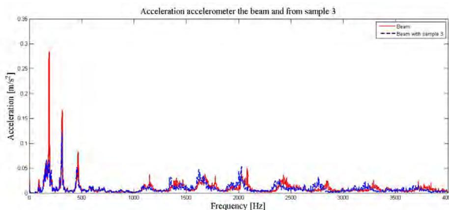
Figure 8. Comparison between frequency response of the beam with sample 3, in terms of acceleration induced by noise white.
