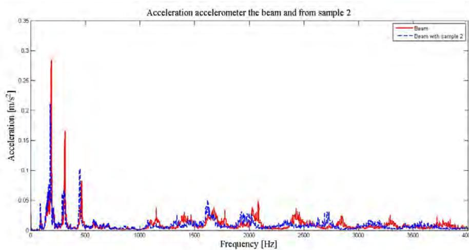
Figure 6. Comparison between frequency response of the beam with sample 2, in terms of acceleration induced by noise white.
