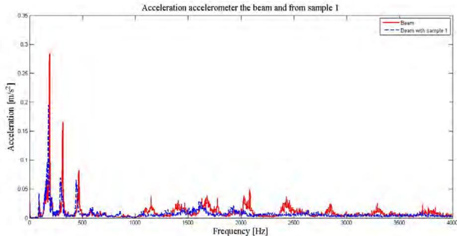
Figure 4. Comparison between frequency response of the beam with sample 1, in terms of acceleration induced by noise white.
