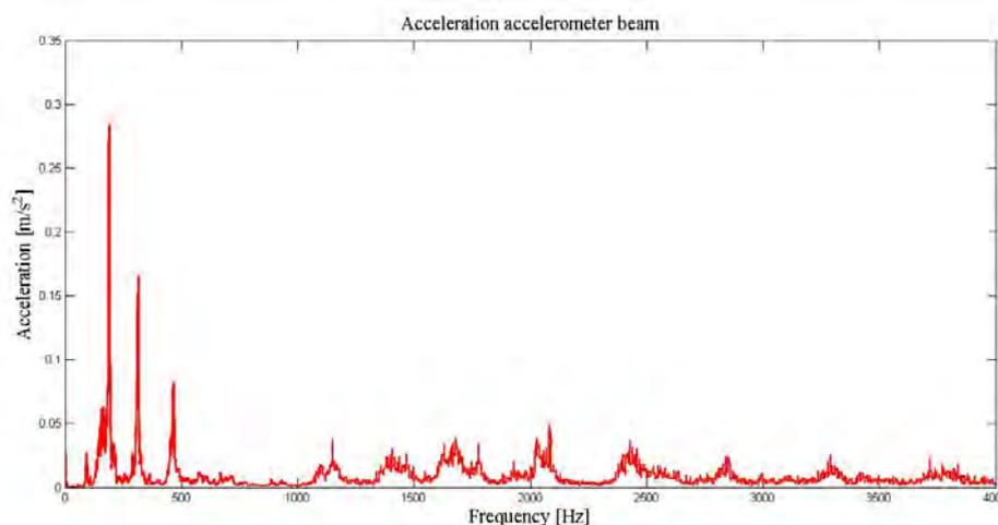
Figure 2. Frequency response of the beam in terms of acceleration induced by noise white.
