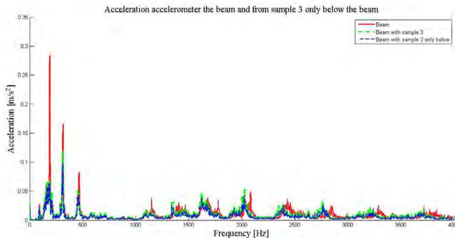
Figure 10. Comparison between frequency response of the beam with sample 3 only below of the beam, in terms of acceleration induced by noise white.
