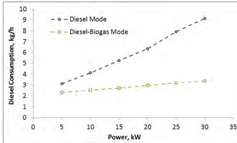
Figure 6. Diesel consumption in diesel mode and in dual mode.
