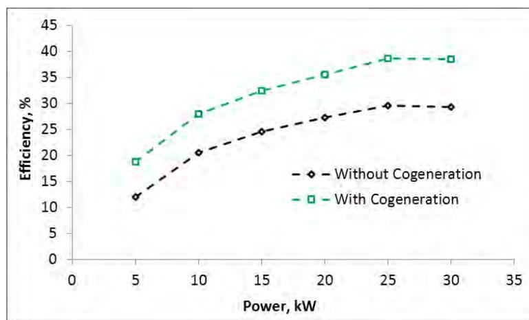
Figure 9. Power generation efficiency and total efficiency of the microgenerator.
