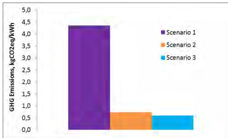
Figure 10. GHG emissions per kWh produced for the three different scenarios.
