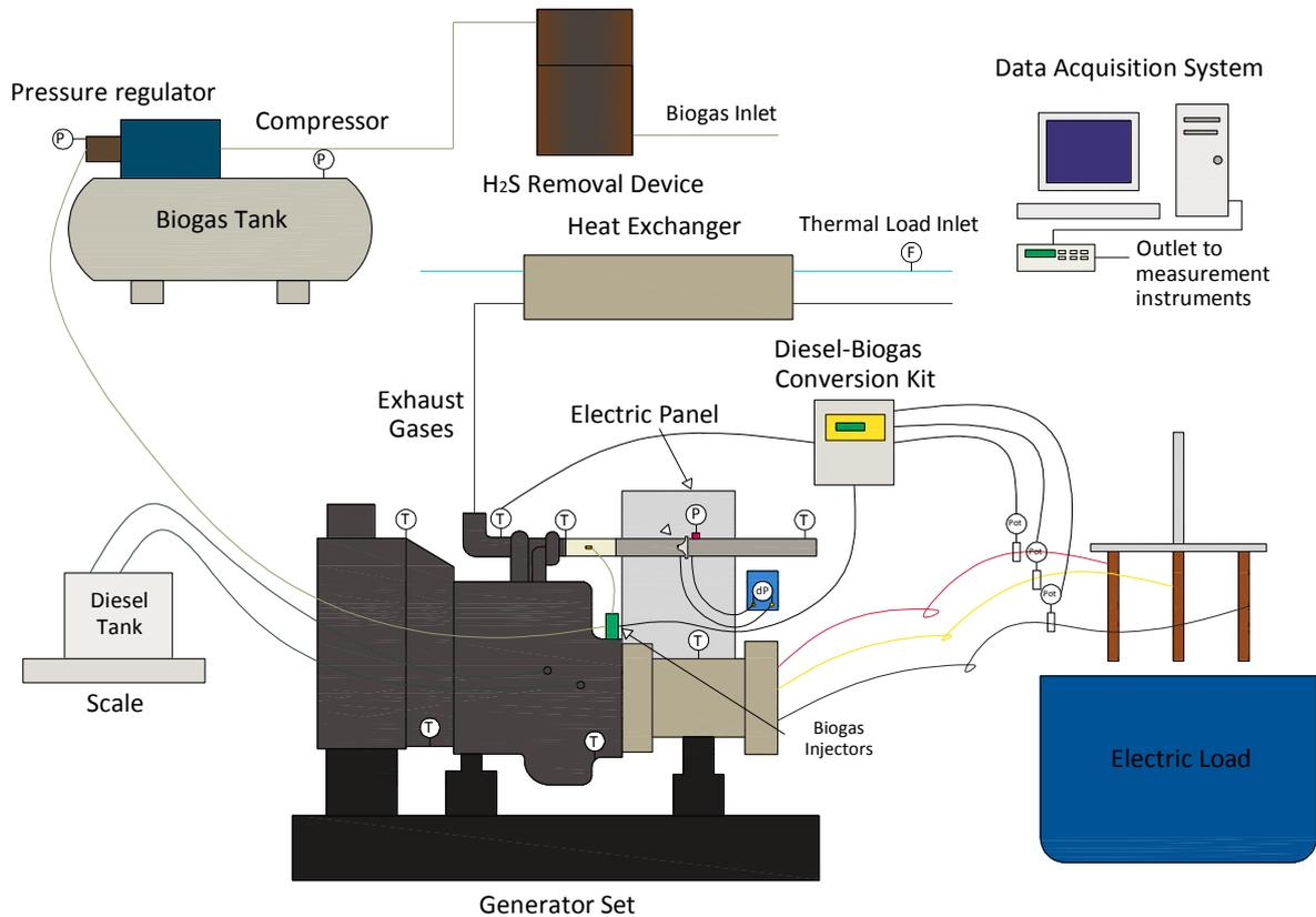
Figure 1. Schematic diagram of the experimental model.
