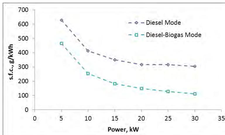
Figure 7. Specific diesel fuel consumption in diesel mode and dual mode.
