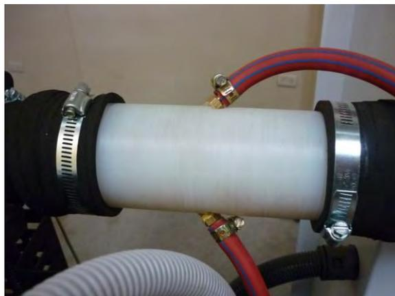
Figure 3. Cylindrical air-biogas mixing device.
