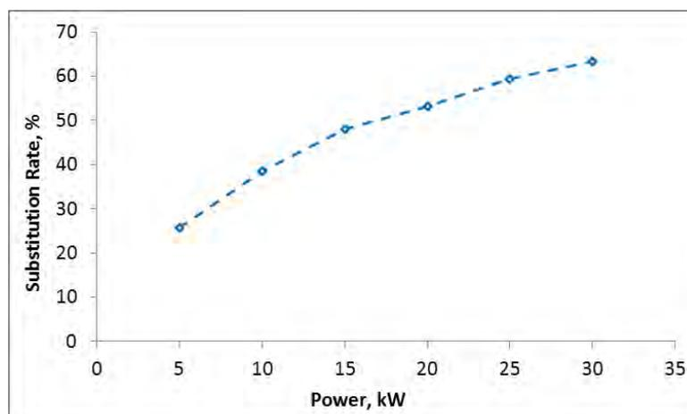
Figure 5. Diesel substitution rates.
