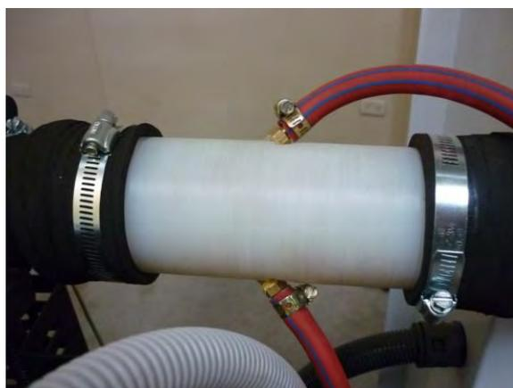
Figure 3. Cylindrical air-biogas mixing device.
