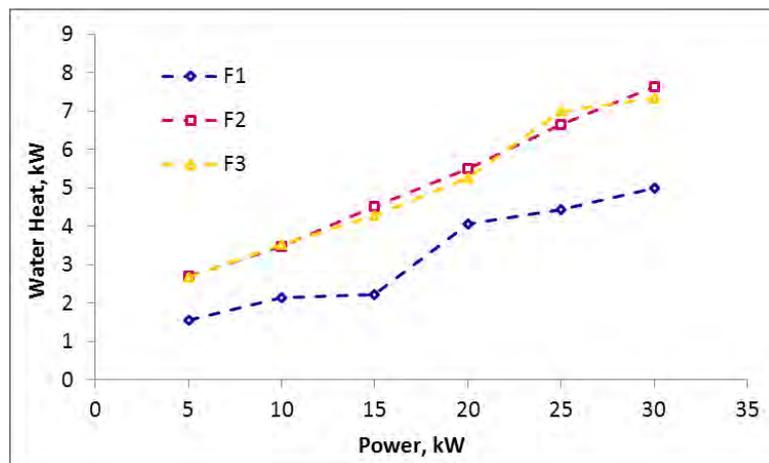
Figure 8. Energy recovered by the water from the exhaust gases.
