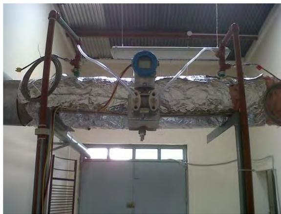
Figure 4. Instrumented heat exchanger.
