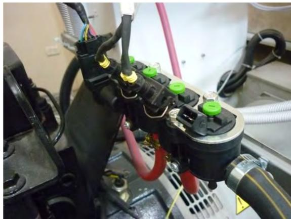
Figure 2. Biogas injectors.
