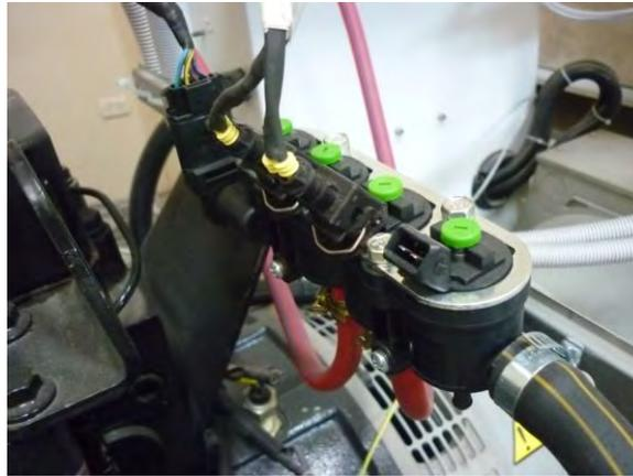
Figure 2. Biogas injectors.
