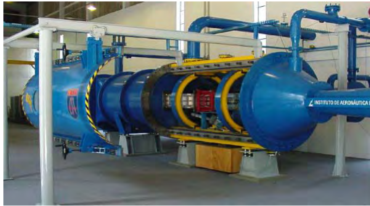
Figure 1. Pilot Transonic Wind Tunnel installation.
