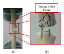
Figure 10- Tensile test on sutured sample. (a) sample placed between the grips (b) enlargement at region highlighting the tearing of the tissue.
