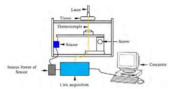
Figure 4- Schematic drawing of experimental apparatus used to measure the temperature along skin.
