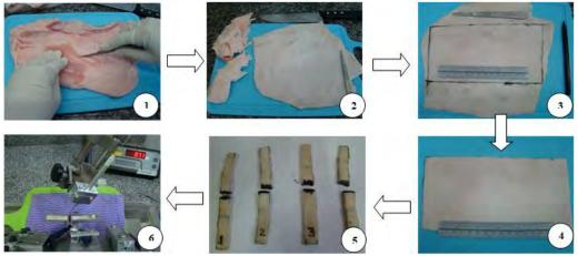
Figure 3 - Flowchart of the process preparation to laser tissue welding process.
