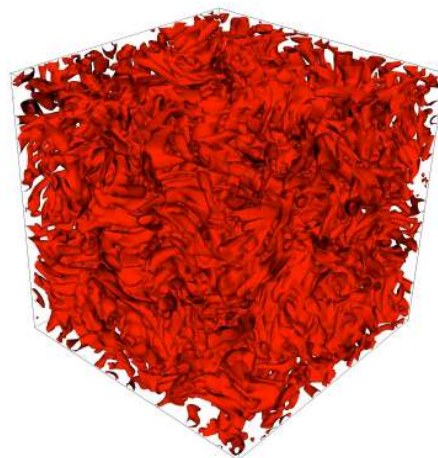
Figure 4: Instantaneous visualization of the enstrophy distribution in a compressible, homogeneous isotropic turbulent field. Data courtesy of Eric Johnsen, Michigan Institute for Plasma Science and Engineering.
