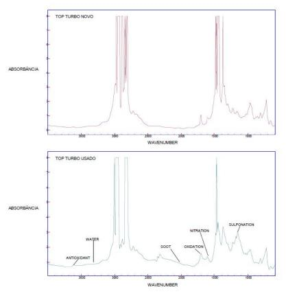
Figure 3. Infrared for the Oil of Engine MWM01
