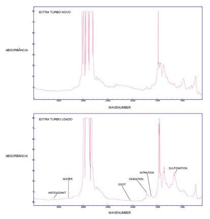
Figure 4. Infrared for the Oil of Engine MWM02
