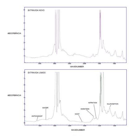
Figure 5. Infrared for the Oil of Engine MWM03
