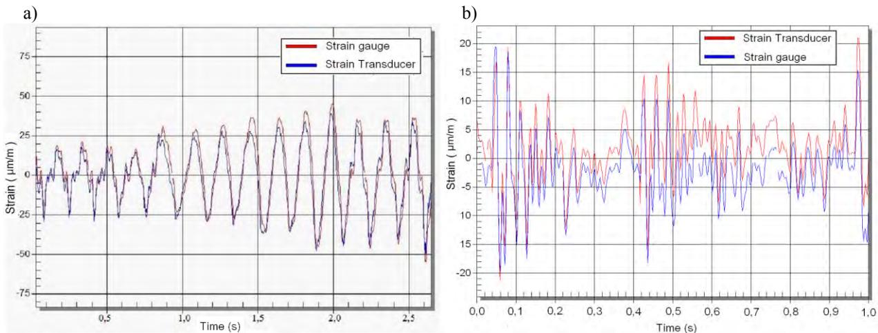
Figure 7 - Comparison between the strain measured by the transducer and a strain gage: (a) Prototype 01 and (b) prototype 03
