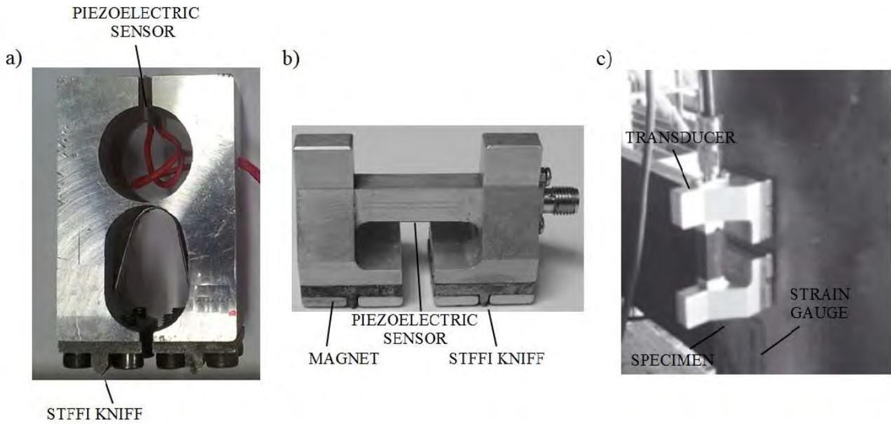
Figure 6. Strain transducer photographs: (a) Transducer with configuration 01, (b) Transducer with configuration 03 and (c) Transducer under testing.
