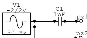
Figure 8. Simplified electrical model of a piezoelectric sensor.
