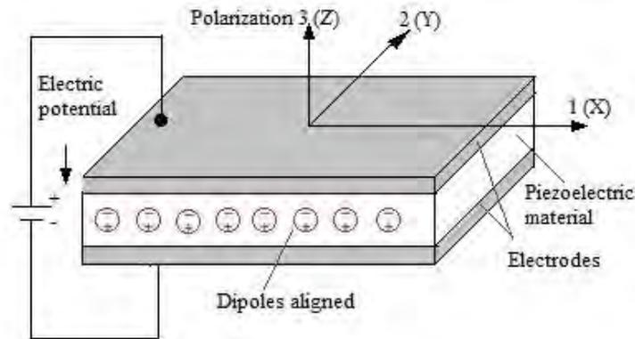
Figure 1. PZT Configuration Direction and orientation axis of piezoelectric material
