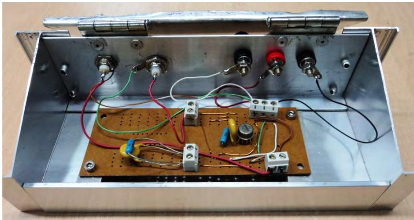
Figure 10. Experimental amplifier with low cut frequency ( Farias, 2013).
