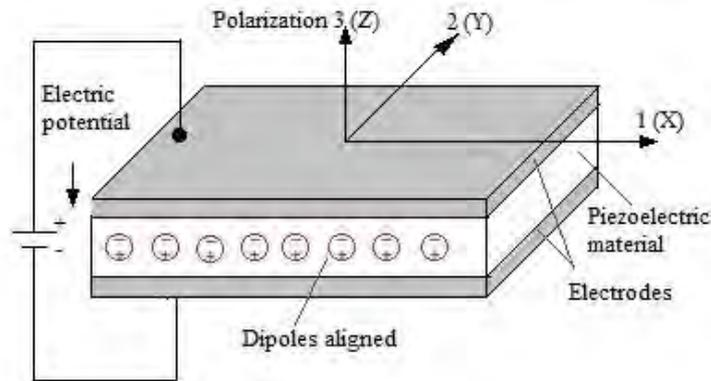
Figure 1. PZT Configuration Direction and orientation axis of piezoelectric material
