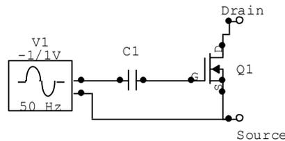
Figure 12. Piezoelectric sensor connected to a depletion MOSFET.
