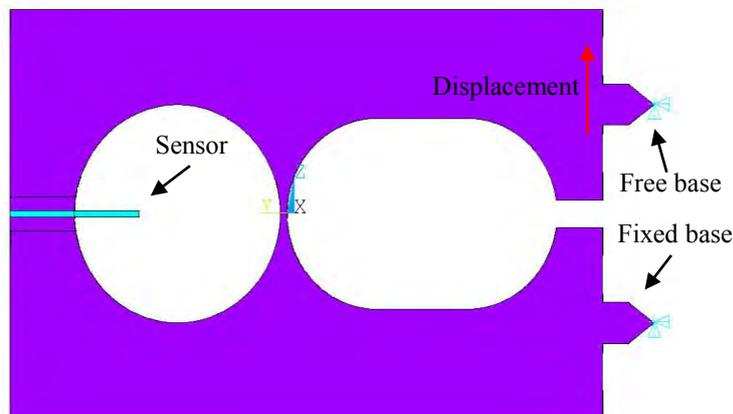
Figure 3. Specimen of transducer in the ANSYS
