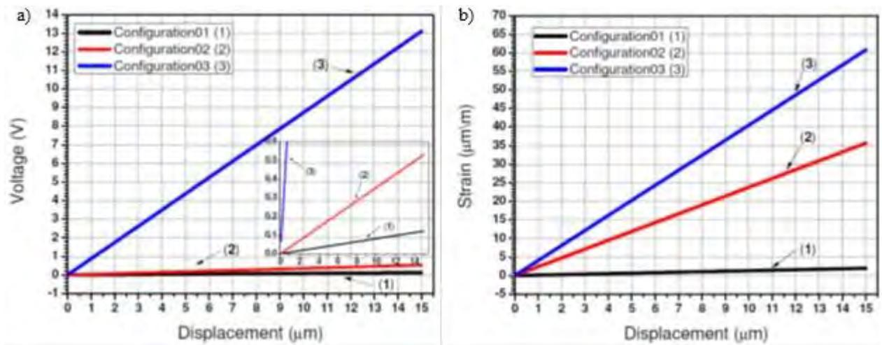
Figure 5. Transducer's sensibility as a function of displacement for each configuration: (a) Voltage; (b) Strain
