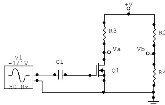
Figure 13. Displacement detection using  $R_{ds}$  as part of a wheatstone bridge circuit.
