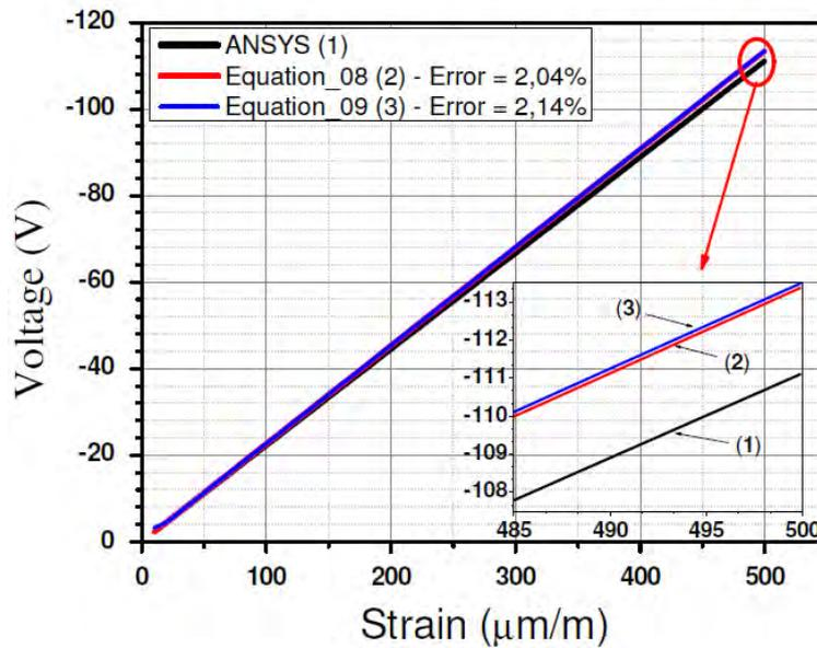
Figure 4. Voltage *versus* strain is extensional displacement of the sensor
