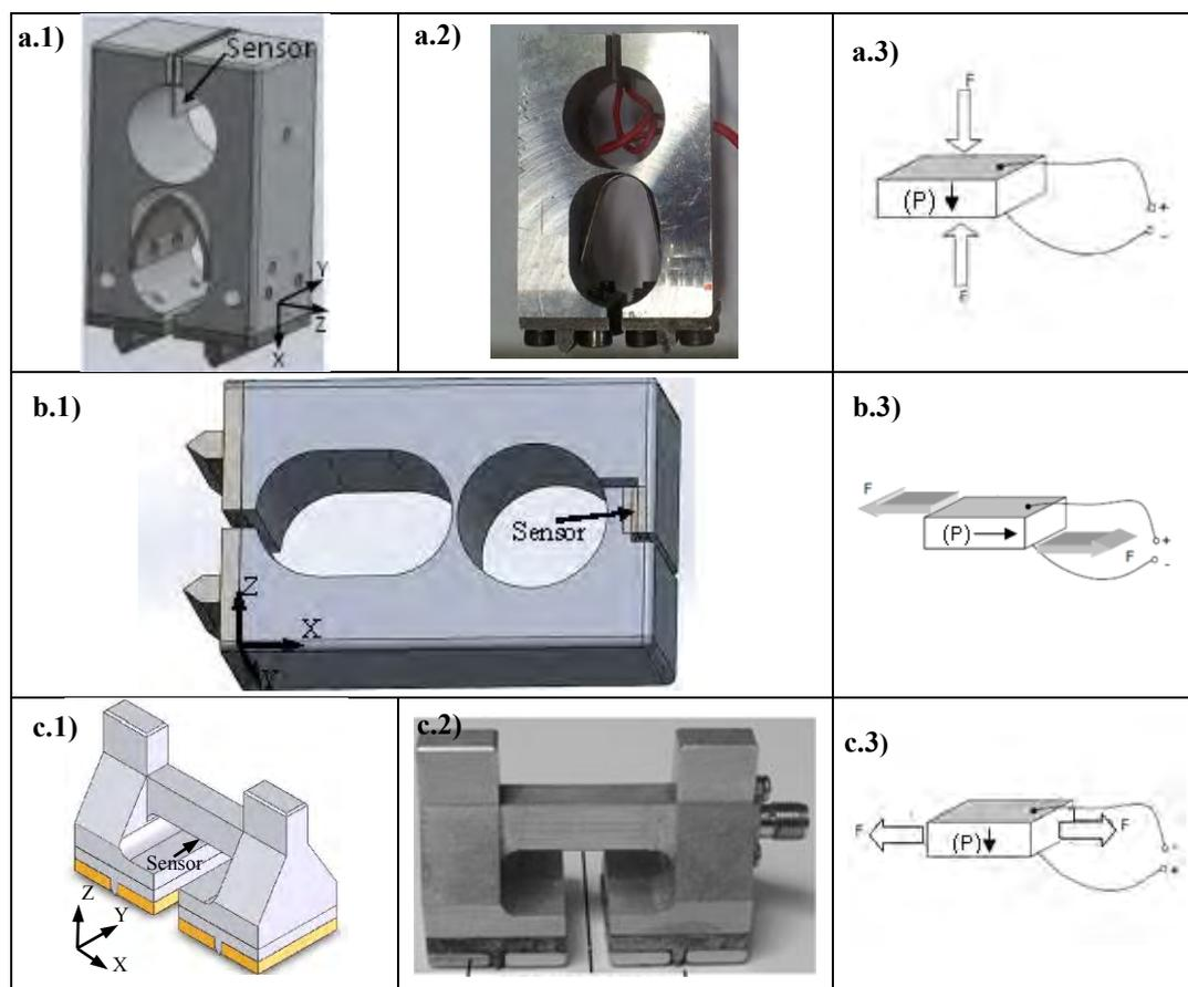
Figure 2. Piezoelectric transducers. (a.1), (b.1) e (c.1): configuration 01, 02 e 03, respectively; (a.2) and (c.2): photograph of the prototype; (a.3), (b.3) e (c.3): Piezoelectric sensor operation modes Longitudinal ( $d_{33}$ ), Shear ( $d_{15}$ ) and extensional ( $d_{31}$ ), respectively.
