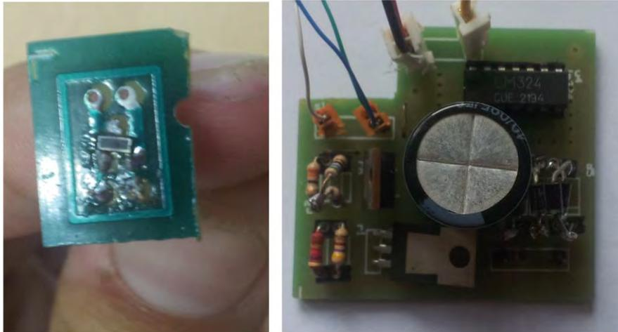
Figure 15. Mosfet (left) and constant current source (right).
