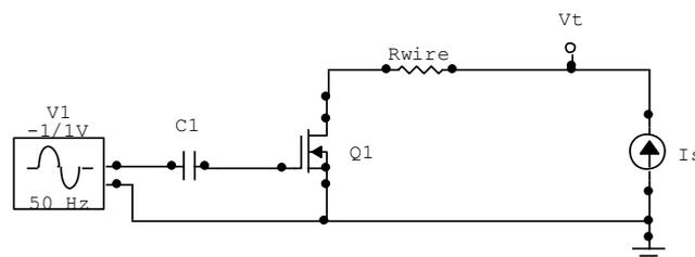
Figure 14. Displacement detection using  $R_{ds}$  with a constant current source.
