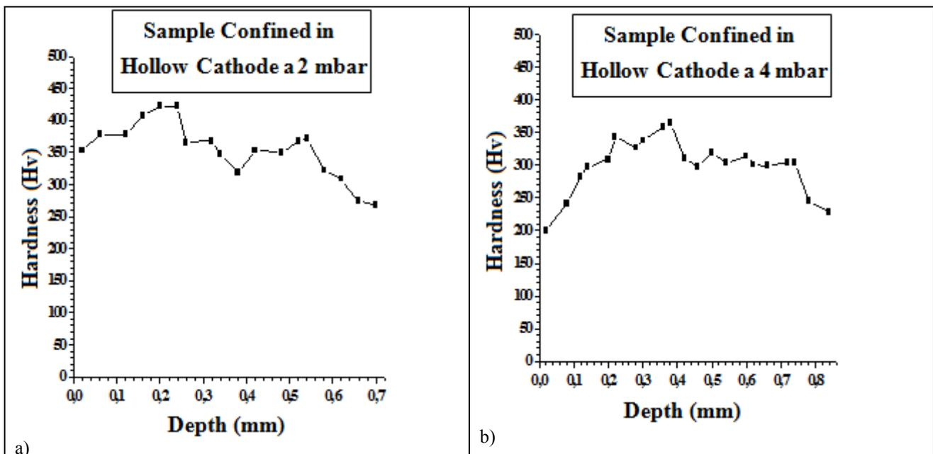
Figure 4 – Profiles of the hardness values the samples in cross-section along their depth. Central region. - (a, b) Profiles samples tempered in plasma by configuration hollow cathode in a pressure of 2 and 4 mbar, respectively.
