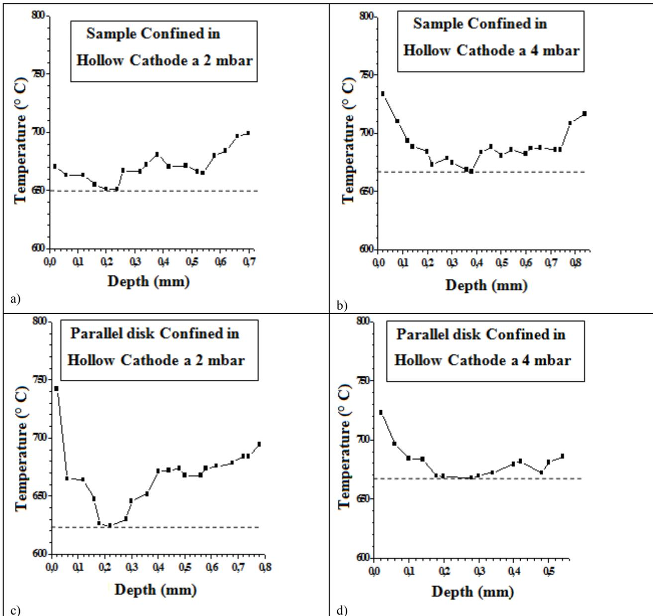
Figure 7 - Profiles of temperature values the samples in cross-section along their depth. Central region. - (a, b) Profiles of samples tempered in plasma by hollow cathode configuration in a pressure of 2 and 4 mbar, respectively. - (c, d) Profiles of disks parallel tempered in plasma by configuration hollow cathode at a pressure of 2 and 4 mbar, respectively.
