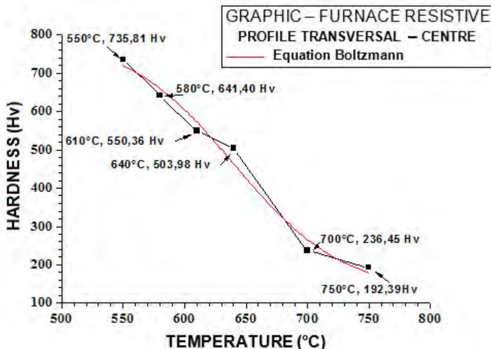
Figure 3 - Curve hardness versus tempering temperature for samples treated in resistive furnace.
