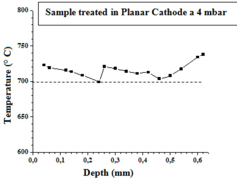
Figure 9 - Thermal profile in the cross section of the sample tempered in plasma by cathode planar configuration, the pressure of 4 mbar along their depth. Central region.
