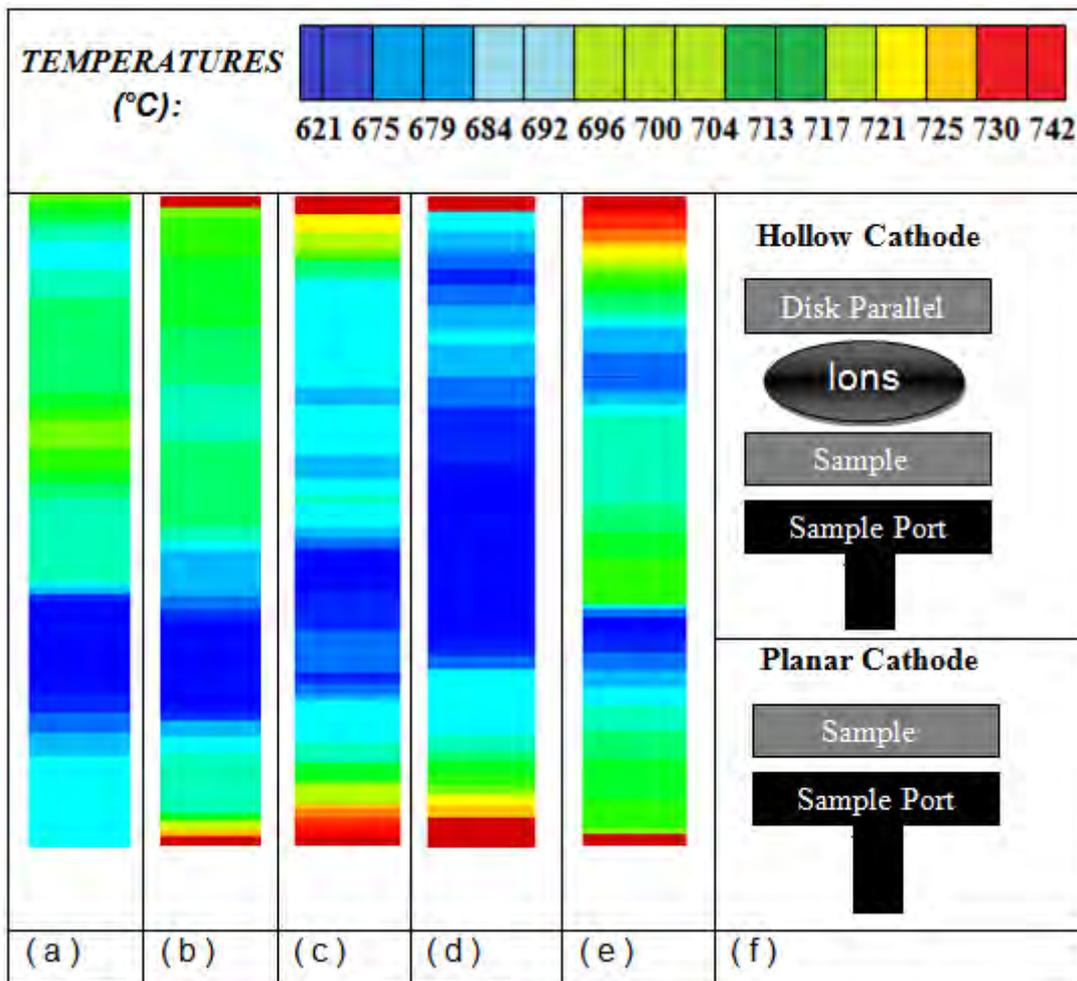
Figure 10 - Behaviour of the temperature profile along the cross section of the samples treated in plasma, where: (a) Sample confined the 2mbar, (b) parallel disc confined the 2mbar (c) Sample confined the 4mbar (d) parallel disc confined the 4mbar (e) Sample treated in planar plasma the 4mbar.
