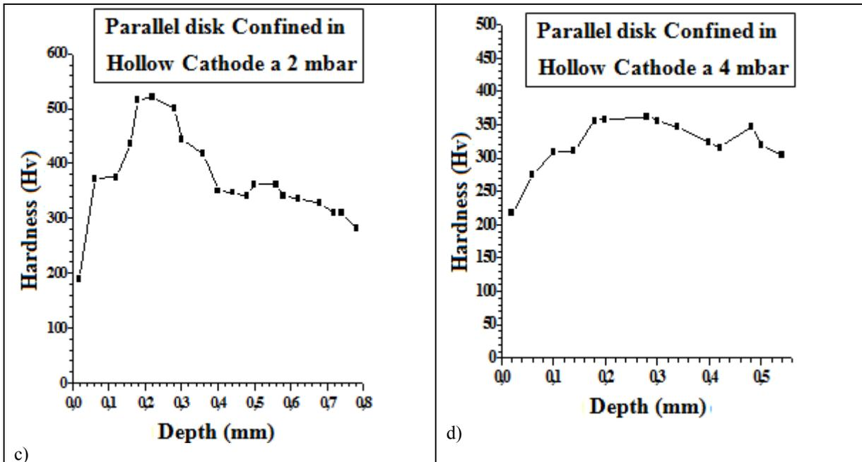
Figure 5 – Profiles of the hardness values the samples in cross-section along their depth. Central region. - (c, d) Profiles of the disks parallel tempered in plasma by configuration hollow cathode at a pressure of 2 and 4 mbar, respectively.
