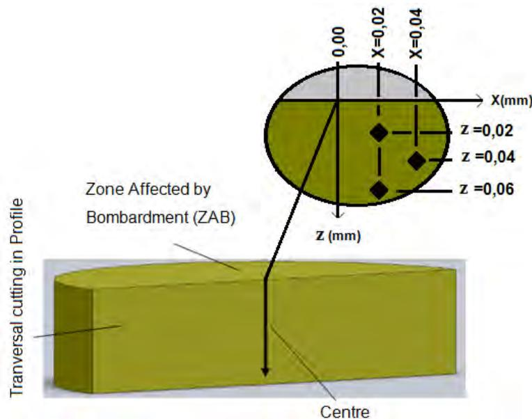
Figure 2 – Representation of the profile cutting of the sample, indicating the region and the direction, in which the microhardness essays were performed.
