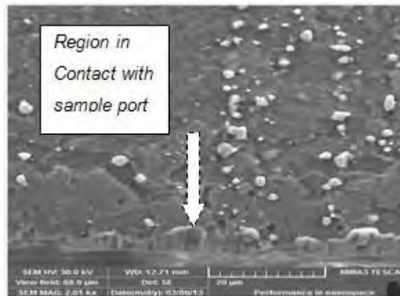
Figure 8 - Micrograph of the sample tempered in plasma and confined at a pressure of 2 mbar showing micro welds obtained with the scanning electron microscope (SEM). Increase of 2000 times.
