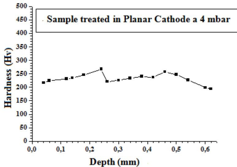
Figure 6 - Profile of hardness in the cross section of the sample tempered in plasma by cathode planar configuration, in the pressure of 4 mbar along their depth (central region).
