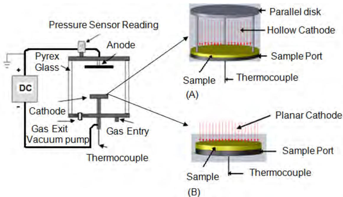
Figure 1 - Schematic plasma equipment used for tempered the steel discs of quenched steel AISI M35. (A) Configuration Hollow Cathode, (B) Configuration Planar cathode.
