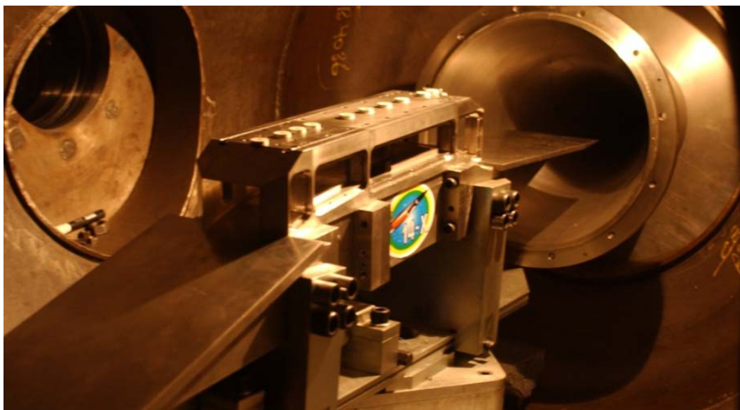
Figure 14: Instrumented truncated 14-X waverider scramjet model installed at the T3 Hypersonic Shock Tunnel.
