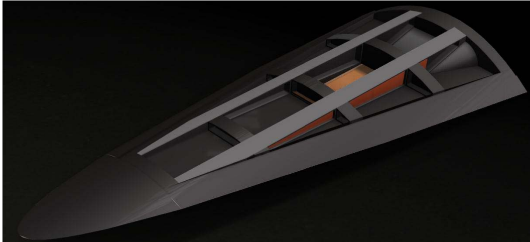
Figure 19: 14-X waverider scramjet internal configuration.
