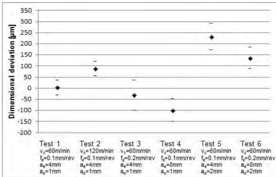
Figure 9. Effect of cutting conditions on dimensional deviation (milled width).
