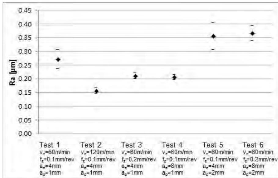
Figure 11. Effect of cutting conditions on surface roughness  $R_a$ .
