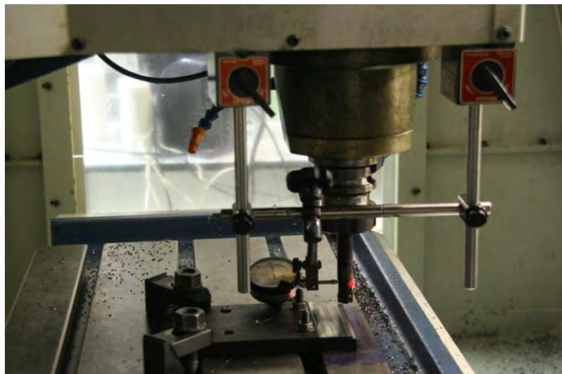
Figure 3. Calibration of the measurement system.
