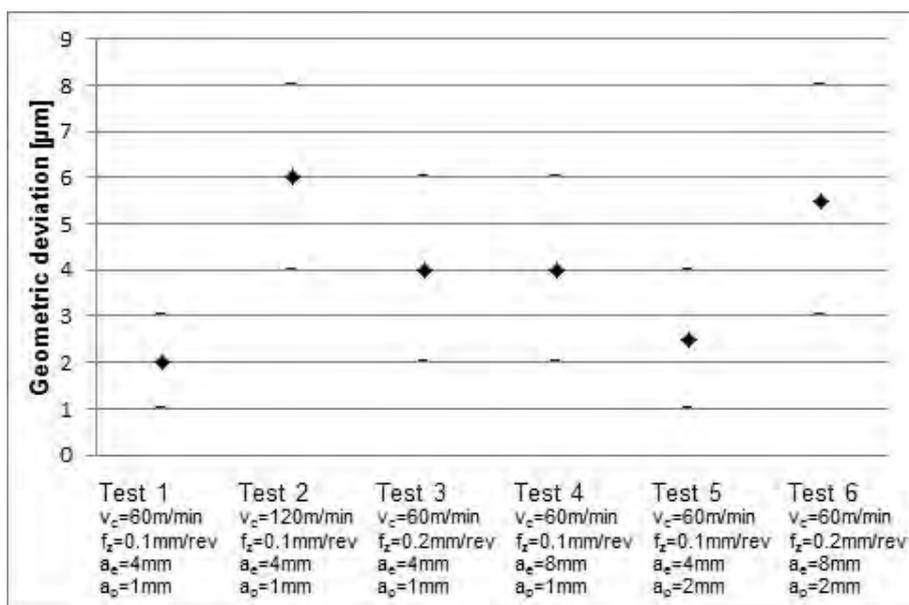
Figure 10. Effect of cutting conditions on machined surface flatness.
