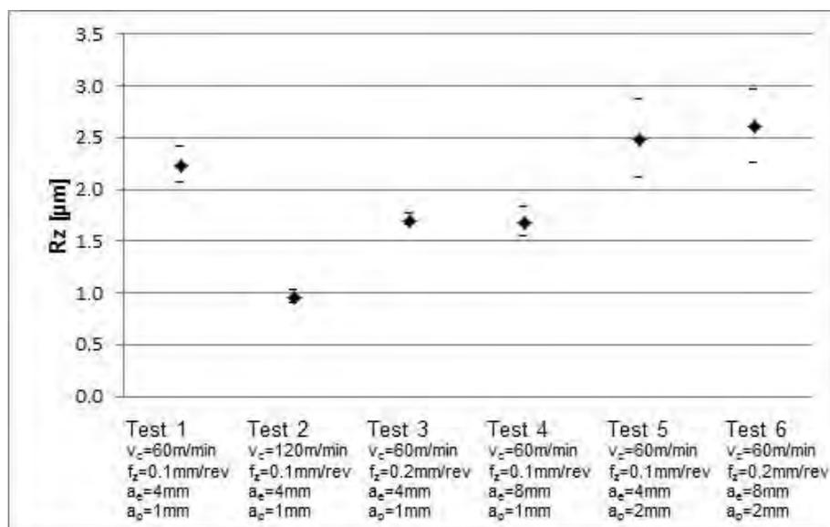
Figure 12. Effect of cutting conditions on surface roughness  $R_z$ .
