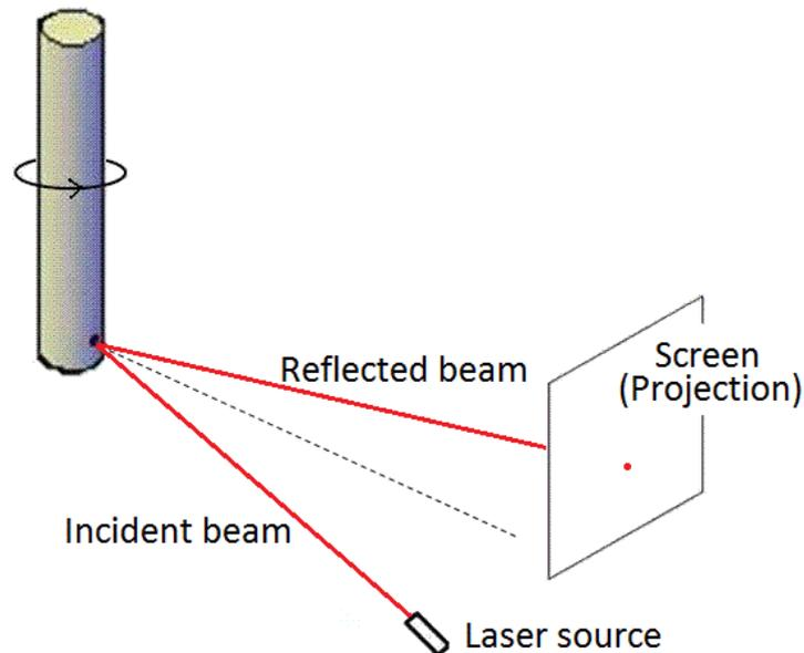
Figure 2. Principle of laser triangulation.
