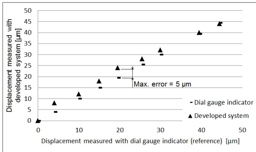
Figure 4. Tool deflection measured by the developed system and by the dial gauge indicator.
