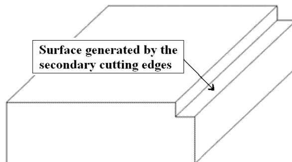
Figure 7. Surface generated by secondary cutting edges.
