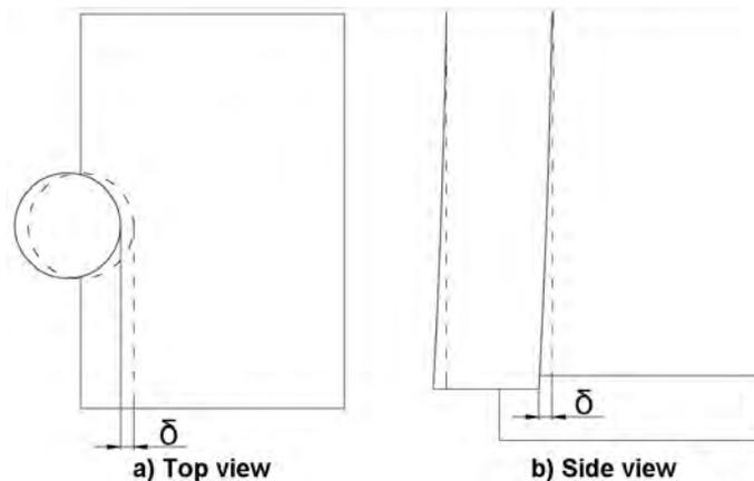
Figure 6. Dimensional deviation of the milled width.
