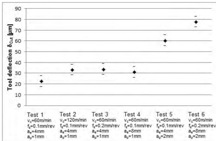
Figure 8. Effect of cutting conditions on cutting deflection  $\delta_{Cut}$ .
