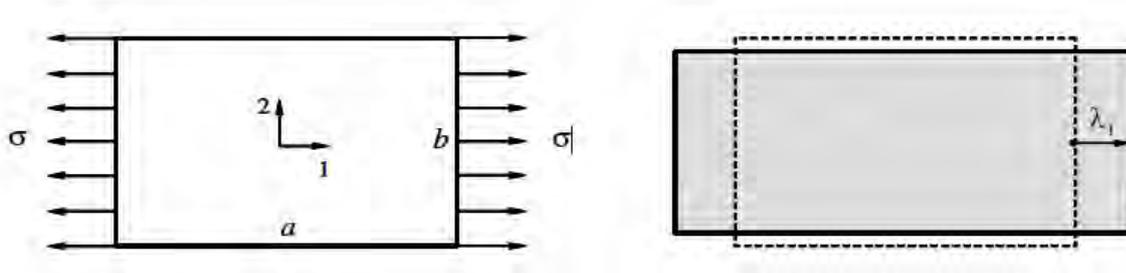
Figure 1. Axial tension of an incompressible sheet
