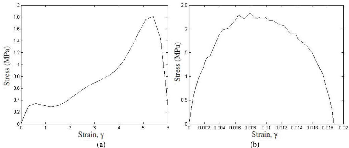
Figure 3. Dissipated energy between loading and unloading: (a) Natural rubber loaded to the maximum stress curve of Fig. 1; (b) PPC7712
