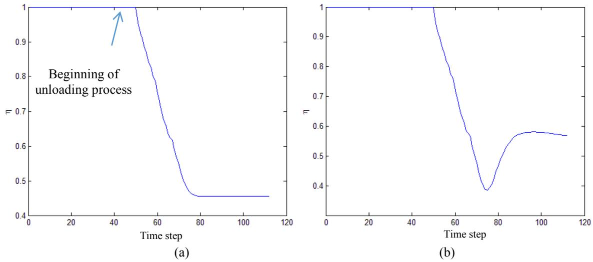
Figure 6. Variation of  $\eta$  in function of the time step for Latex using HMHSI. (a) results for Dorfmann's model, (b) results for the proposed model from Eq. (4.6)
