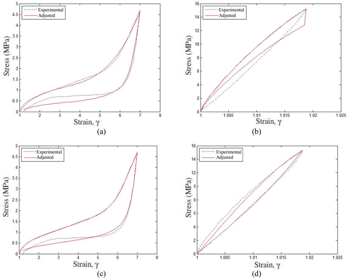
Figure 5. Adjusted data for models HMLSI and HMHSI using Eq. (11): (a) Latex using HMLSI. (b) PPC7712 using HMLSI. (c) Latex using HMHSI. (d) PPC7712 using HMHSI.
