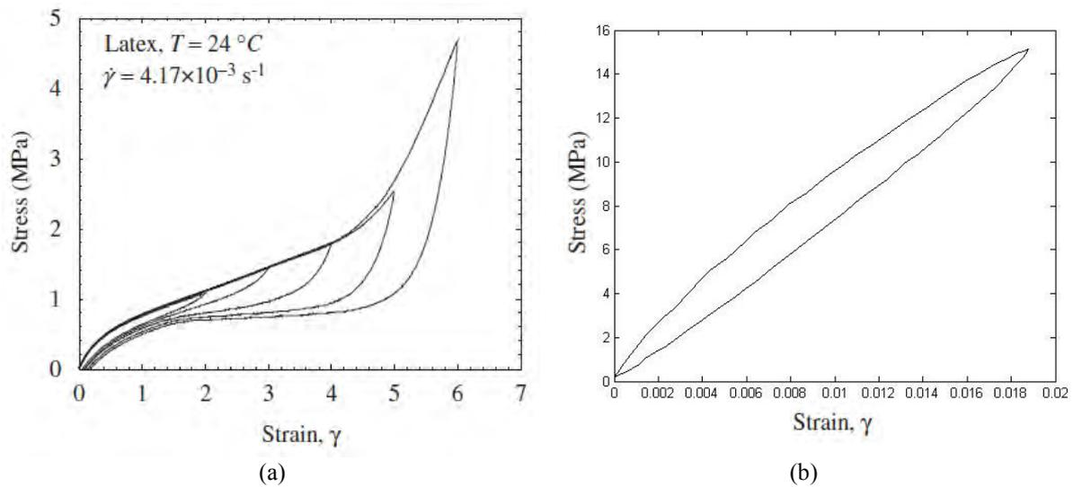
Figure 2. Stress-strain curves: (a) Natural rubber (Niemczura 2011); (b) PPC7712 (Zrida 2009)
