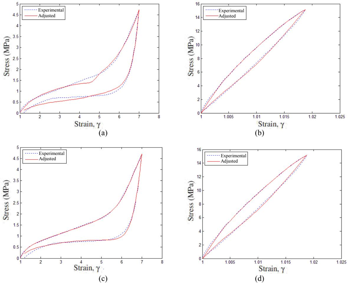
Figure 7. Adjusted data for models HMLSI and HMHSI using Eq. (12): (a) Latex using HMLSI. (b) PPC7712 using HMLSI. (c) Latex using HMHSI. (d) PPC7712 using HMHSI.
