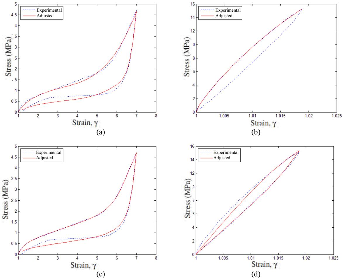
Figure 4. Adjusted data for models HMLSI and HMHSI using Eq. (9): (a) Latex using HMLSI (b) PPC7712 using HMLSI (c) Latex using HMHSI (d) PPC7712 using HMHSI
