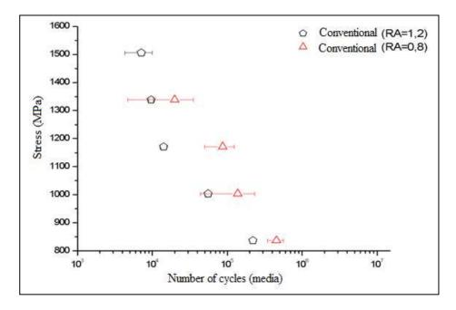
Figure 8. S-logN curves showing the effect of surface roughness on fatigue behavior in axial specimens obtained wire rod produced by conventional casting.
