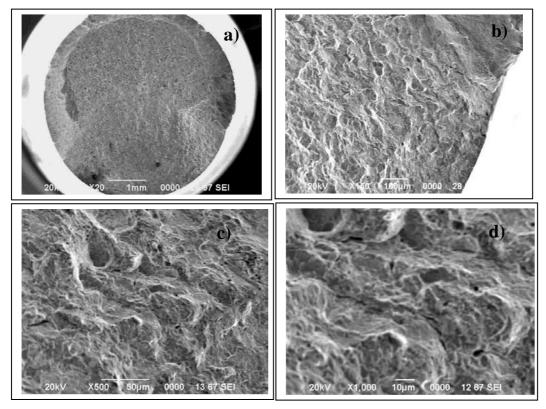
Figure 9. Fracture for 50% of the yield stress, showing the fatigue fracture surfaces with magnifications: 20X (a) 150X (b) 500X (c) 1000X and (d)
