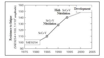
Figure 2. Development of valve springs steels. (SUDA, 2005)
