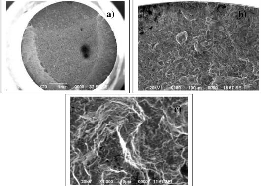
Figure 10. Fracture for 70% of the yield stress, showing the fatigue fracture surfaces with magnifications: 20X (a) 150X (b) 1000X and (c)
