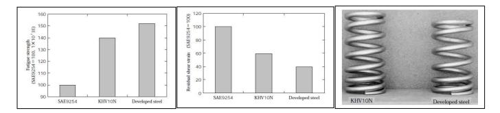
Figure 3. Fatigue strength of steel for valve springs, shear stress residual steel for valve springs and changes in the diameter and number of turns in coil springs valves manufactured with the new generations of steel (SUDA, 2007).
