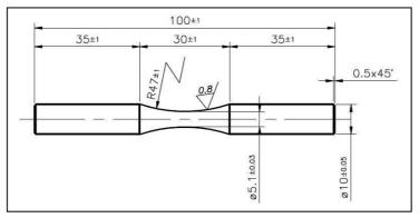
Figure 6. Specimens for axial fatigue test (ASTM E 466)
