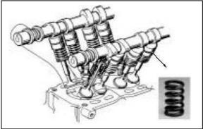
Figure 1. Arrangement of valve springs in an automobile engine (SUDA, 2005)
