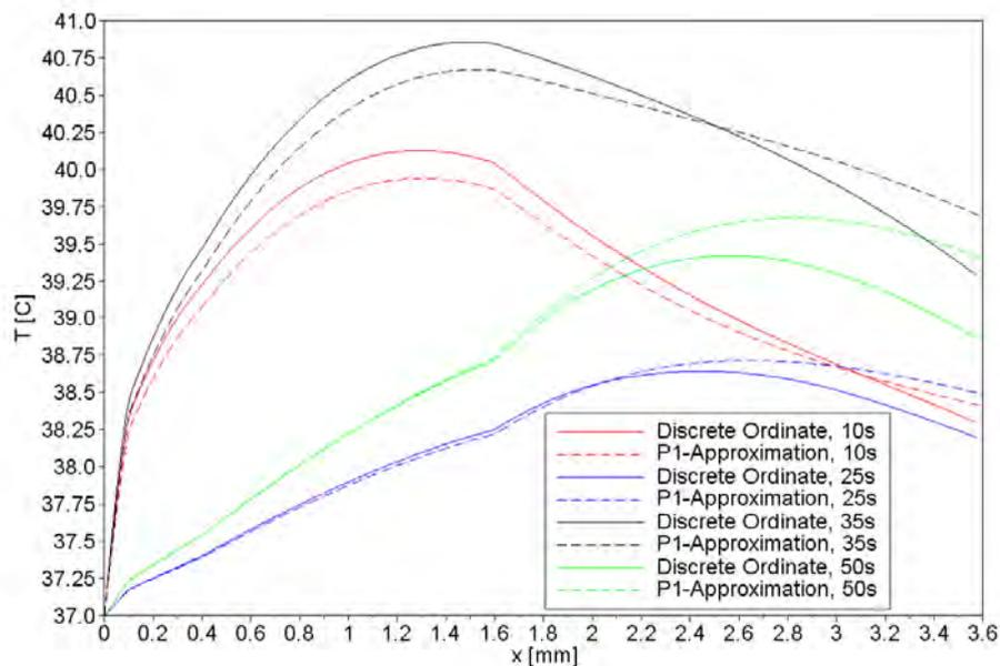
Figure 4 – Comparison of the temperature distribution at computed with the Discrete Ordinate method and the P1-approximation for the tissue without nanoparticles.
