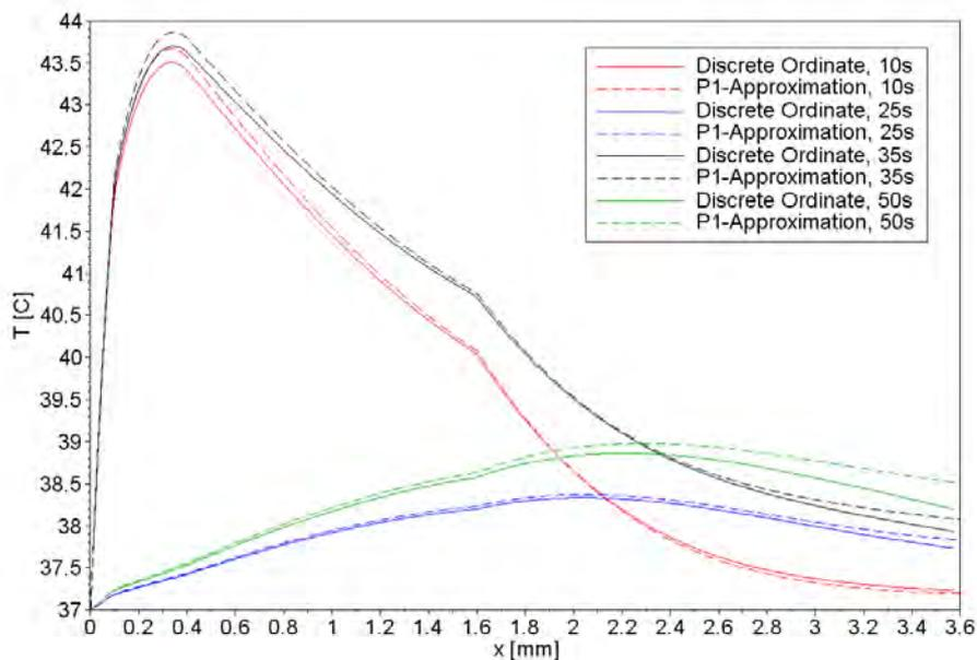
Figure 3 – Comparison of the temperature distribution computed with the Discrete Ordinate method and the P1-approximation for the tissue with nanoparticles.
