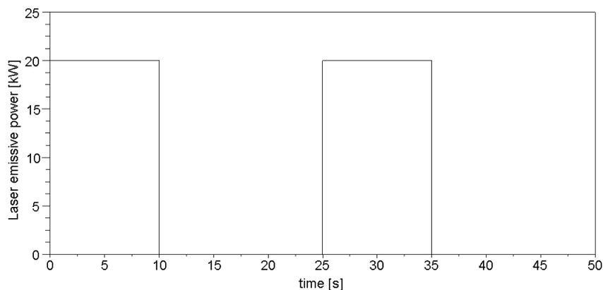
Figure 2 – Variation of the laser emissive power in periodic heating.
