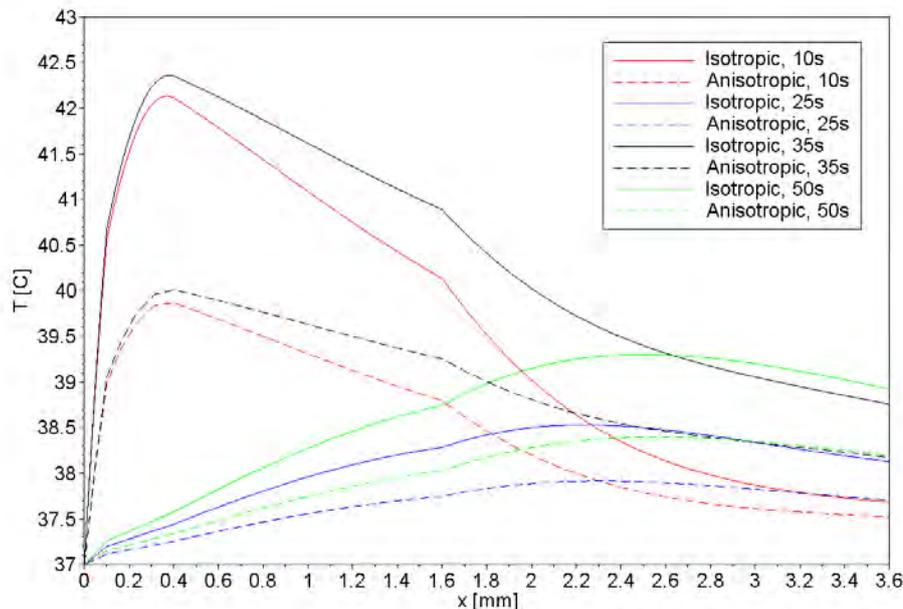
Figure 5 – Comparison of the temperature distribution at different times of exposition to the periodic laser heating for cases of isotropic and anisotropic scattering.
