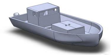
Figure 2. Model chosen: length 11,25 x4, 25 (m), volume of 12.75 urn (m<sup>3</sup>), engine power 94 HP.
