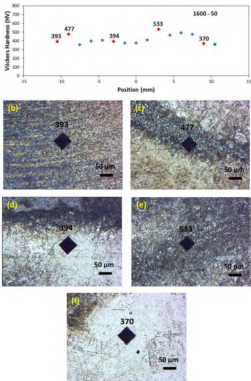
Figure 12 – Vickers hardness as a function of position along transversal direction at condition 7, 1600 RPM and feed 50 mm/min (a);
