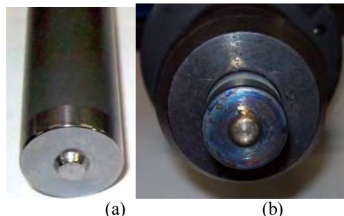
Figure 9 – (a) new tool, (b) tool after FSW.
