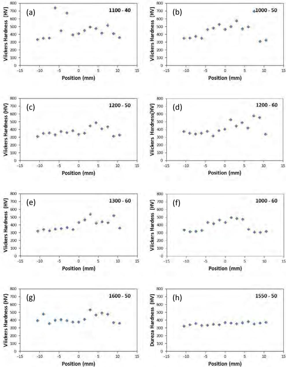
Figure 12 – Vickers hardness as a function of position along transversal direction at conditions 1, 1100 RPM and feed 40 mm/min (a); 2, 1000 RPM and feed 40 mm/min (b); 3, 1200 RPM and feed 50 mm/min (c); 4, 1200 RPM and feed 60 mm/min (d); 5, 1300 RPM and feed 60 mm/min (e); 6, 1000 RPM and feed 60 mm/min (f); 7, 1600 RPM and feed 50 mm/min (g); 8, 1550 RPM and feed 50 mm/min (h).
