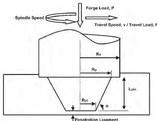
Figure 5 – Basic geometry for FSW tool (EDWARDS e RAMULU, 2009).
