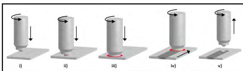
Figure 3 – FSW process steps (MASHININI, 2010).
