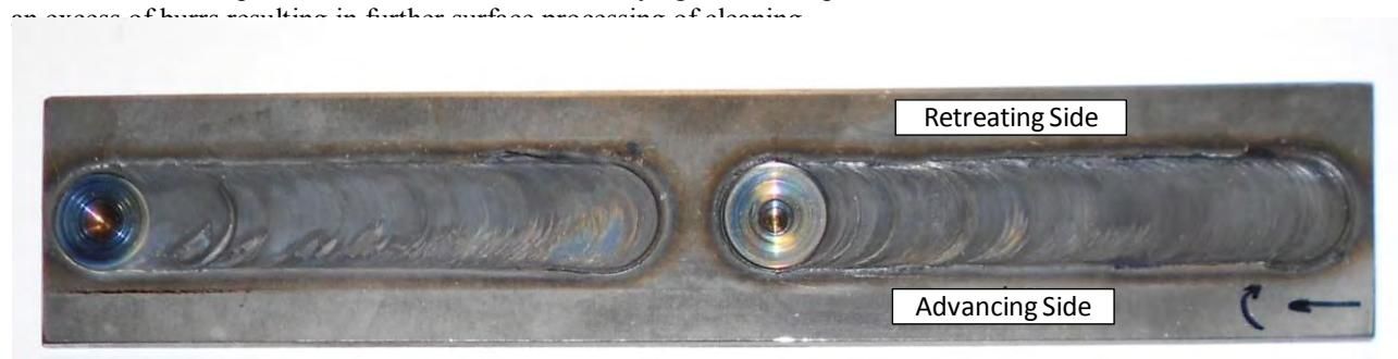
Figure 10 – Sample Ti-6Al-4V (260mmx50mm) after FSW process, AS: advancing side of the tool, RS: retreating side of the tool.
