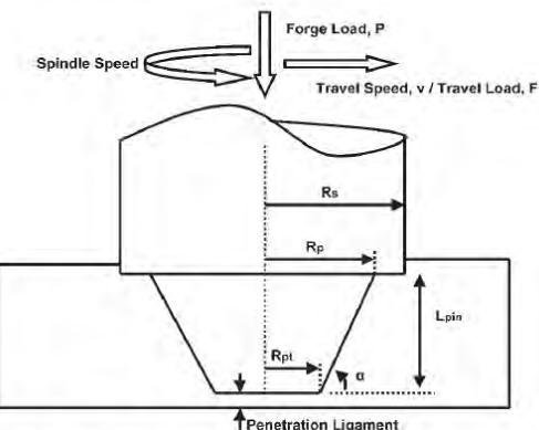
Figure 5 – Basic geometry for FSW tool (EDWARDS e RAMULU, 2009).
