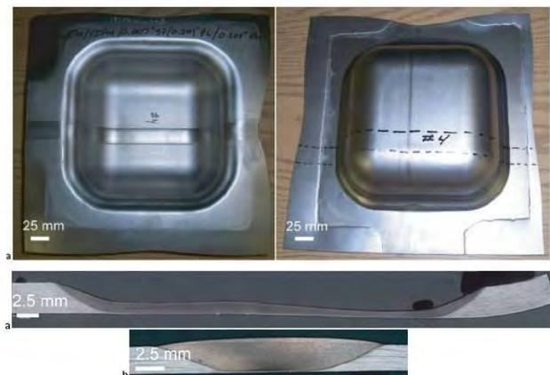
Figure 1 - In (a) processed region is more superplastic than the base material, and (b) the processed region is less superplastic than the base material (EDWARDS e RAMULU, 2009).
