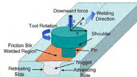
Fig. 1. Schematic drawing of friction stir welding.
