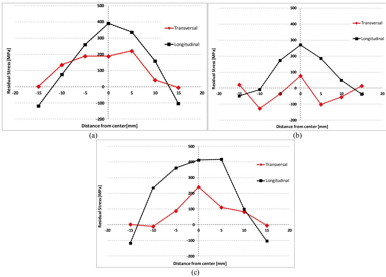
Figure 11 – Residual stress at conditions 1 (a) 1100 RPM and feed 40 mm/min; condition 5 (b) 1000 RPM and feed 40 mm/min and condition 3 (c) 1200 RPM and feed 50 mm/min.
