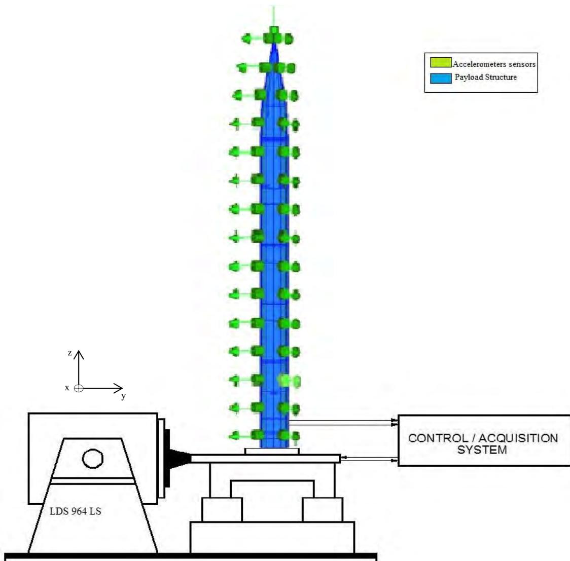
Figure 1. A schematic drawing of the experimental setup.
