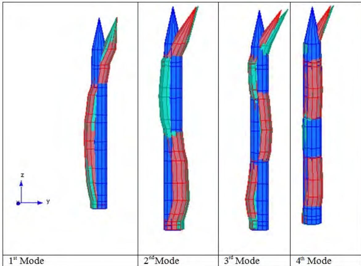
Figure 4. Comparison methods of SSI (in light blue) e EFDD (in red). Dark Blue is related to the static body.
