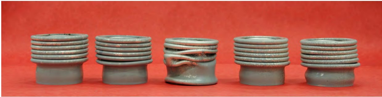
Figure 6: Prototype made of aluminium. Samples 1-5 from left to right. All except sample #3 buckled as concertina or axisymmetric mode. Concertina mode developed 6 folds and left enough length for a seventh.
