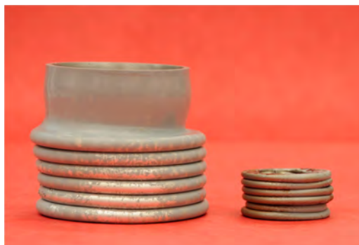
Figure 10: Prototype made of aluminium developed shorter folds than model made of steel ( \beta = 0.50 ). It was expected a similar global aspect since fold length is usually defined as function of geometrical parameters only (Jones, 1997).
