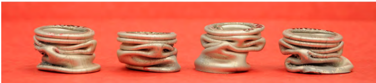
Figure 7: Aluminium models ( \beta = 0.5 ) buckled as diamond mode. The initial compression phase results in two folds in concertina mode, followed by unstable diamond folds.
