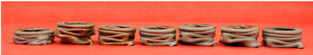
Figure 8: Steel models ( \beta = 0.75 ). All 7 tubes buckled as diamond mode. The last, #7, reach the maximum of 3 concertina folds.
