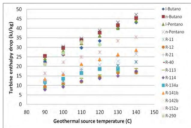
Figure 8. Turbine enthalpy drops for each working fluid at different geothermal source temperature
