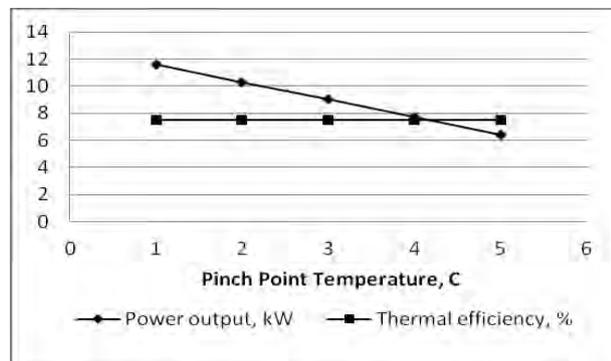
Figure 4. Power output and thermal efficiency of the cycle for different pinch points values.
