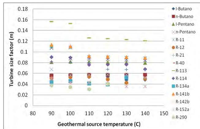
Figure 13. Turbine size factor for each working fluid at different geothermal source temperature.
