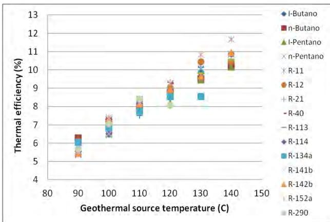
Figure 11. Thermal efficiency for each working fluid at different geothermal source temperature.
