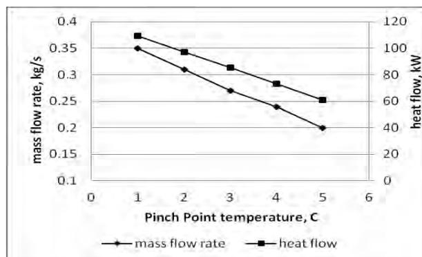
Figure 5. Heat flow and mass flow rate in the evaporator for different pinch points values.
