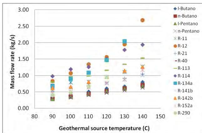
Figure 7. Mass flow rate for each working fluid at different geothermal source temperature.
