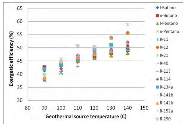
Figure 12. Exergetic efficiency for each working fluid at different geothermal source temperature.
