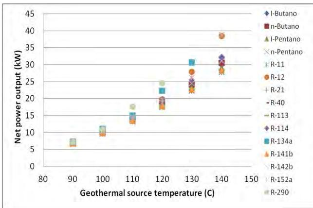
Figure 9. Net power output for each working fluid at different geothermal source temperature.
