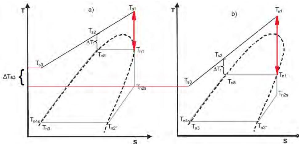
Figure 6. Thermodynamic cycles for the power plant, at the working fluid evaporation temperature  $T_{n1}$  of: a) relatively high value, b) relatively low value.
