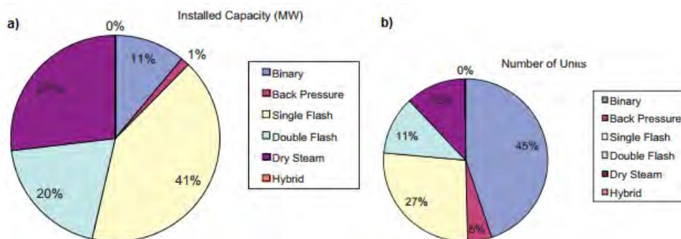
Figure 1. (a) Percentage of installed capacity by power plant type. (b) Percentage of units by power plant type. (Bertani, R., 2012).
