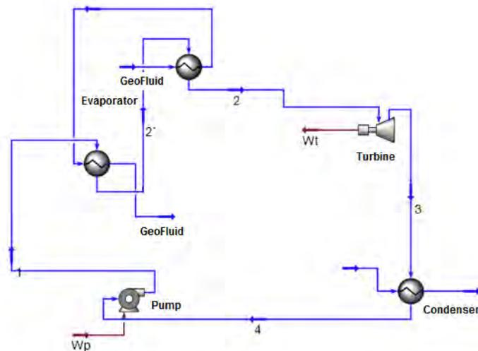
Figure 2. Schematic components of the ORC system for low-enthalpy geothermal source.
