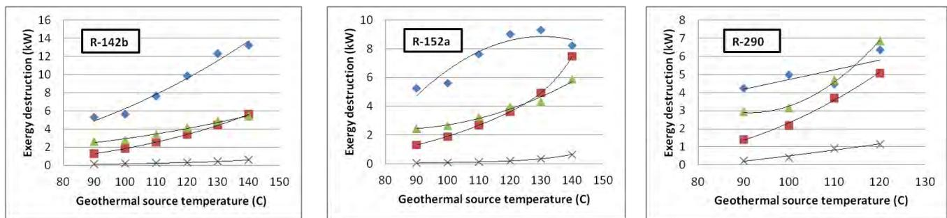
Figure 14. Exergy destruction for the different components and working fluids of the ORC at different geothermal source temperature.
