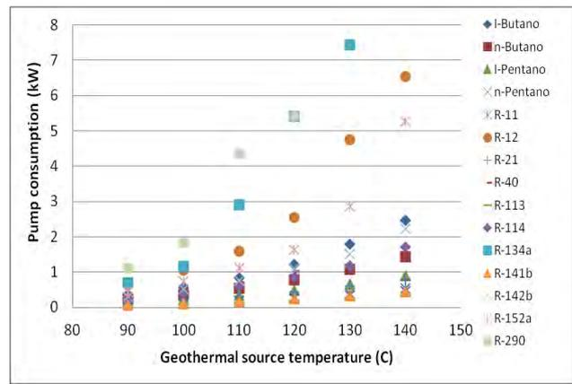
Figure 10. Pump energy consumption for each working fluid at different geothermal source temperature.
