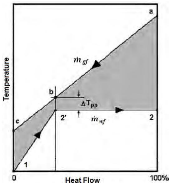
Figure 3. Heat transfer diagram for the evaporator.
