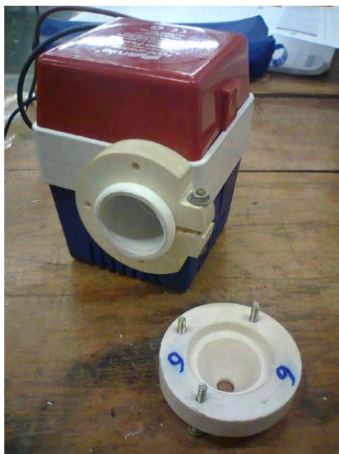
Figure 5. Thrust optimizer and its coupling on a pump.
