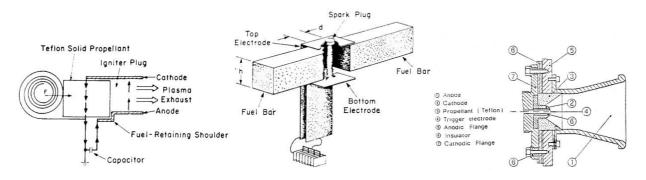
Figure 1. (Gessini et al., 2005) a) (Left) Breech-fed PPT; b) (Center) Side-fed PPT; c) (Right) Coaxial PPT.
