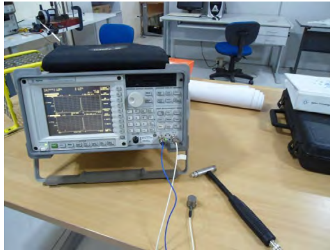
Figure 5. Instrumentation of dynamic signal analysis.
