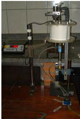
Figure 7. Mechanical model for the measurement of the force provided by the pneumatic actuator
