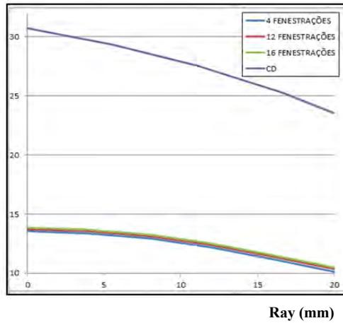
Figure 15. Displacement curve Z (mm) depending on the distance to the center (Ray), comparing with CD to the same 20mm
