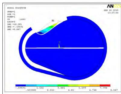
Figure 17. The displacement Y, in the model without a portion of the skull that is removed during surgery, with the maximum point in the dura-mater
