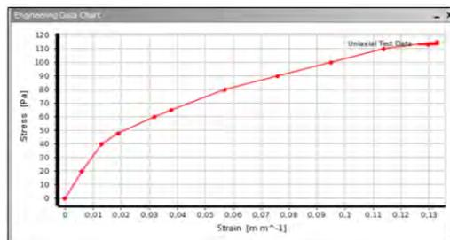
Figure 9. Curve Stress / Deformation obtained in Ansys using the work of Miller
