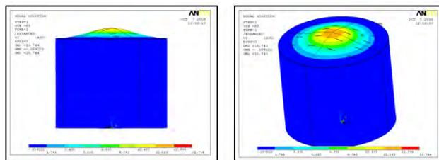
Figure 13. Vertical displacement (Z direction) of the dura-mater with 16 fenestrations
