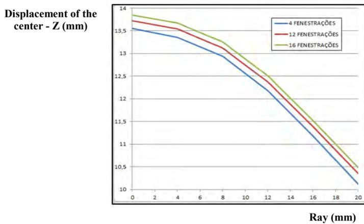
Figure 14. Displacement curve Z (mm) depending on the distance to the center (Ray), showing greater flexibility with more fenestrations
