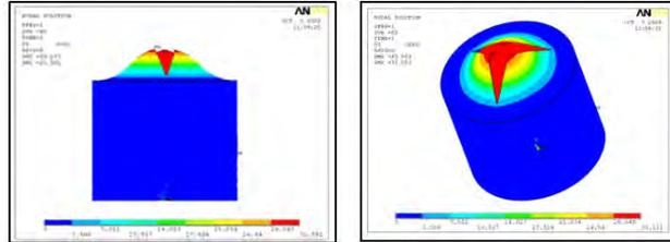
Figure 12. Vertical displacement (Z direction) of the dura-mater in the model used to simulate the DC
