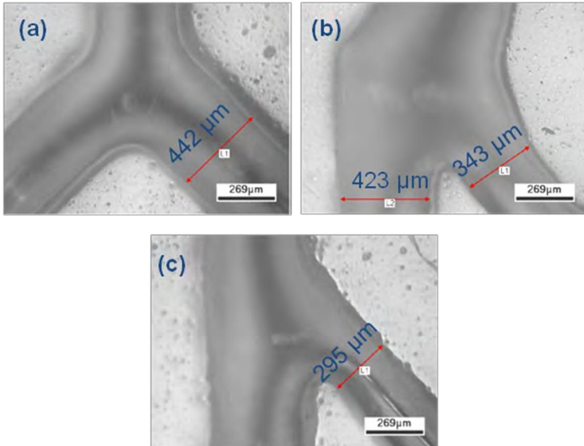
Figure 11 - Image of the Tesla shaped channels by electron microscopy.
