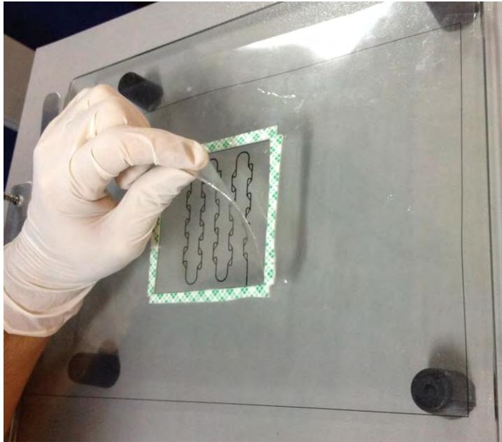
Figure 5 - Removal of the base with the microchannels.
