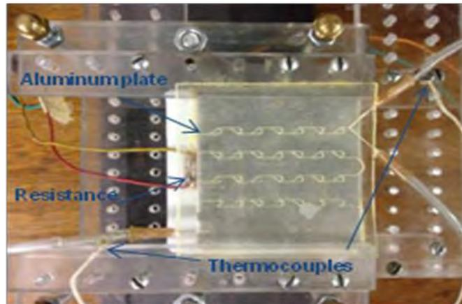
Figure 17 - Details of the support with the micromixer, the resistance and the aluminum plate.
