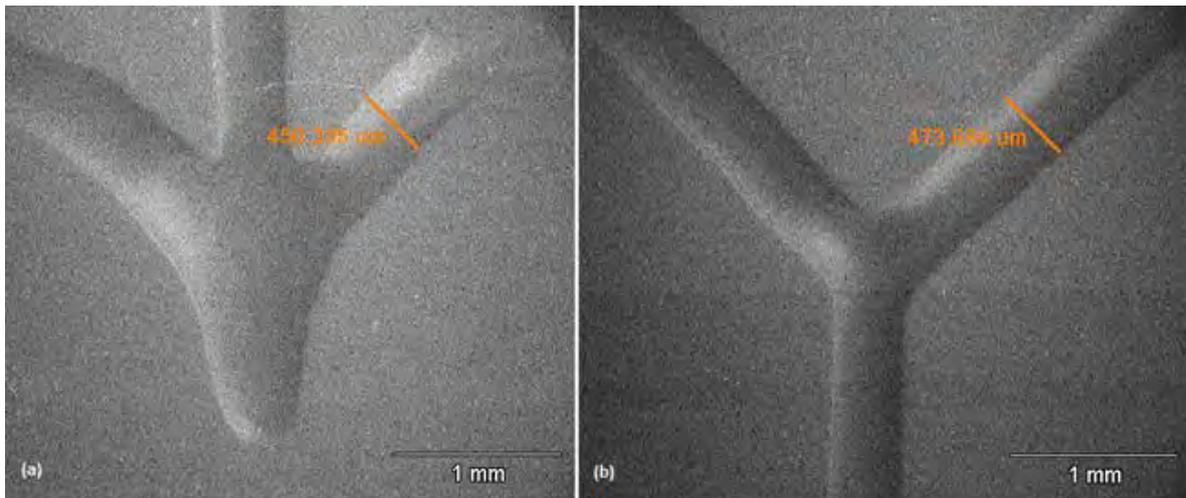
Figure 10 - Images of the Omega shaped channels by electron microscopy.
