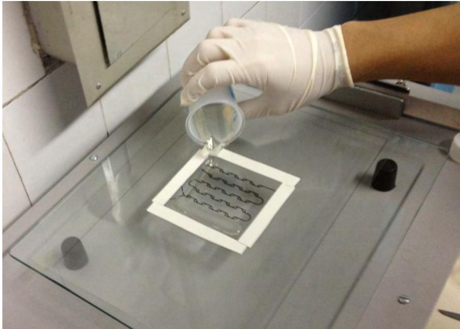
Figure 3 - Preparation and deposition of the photoresist.
