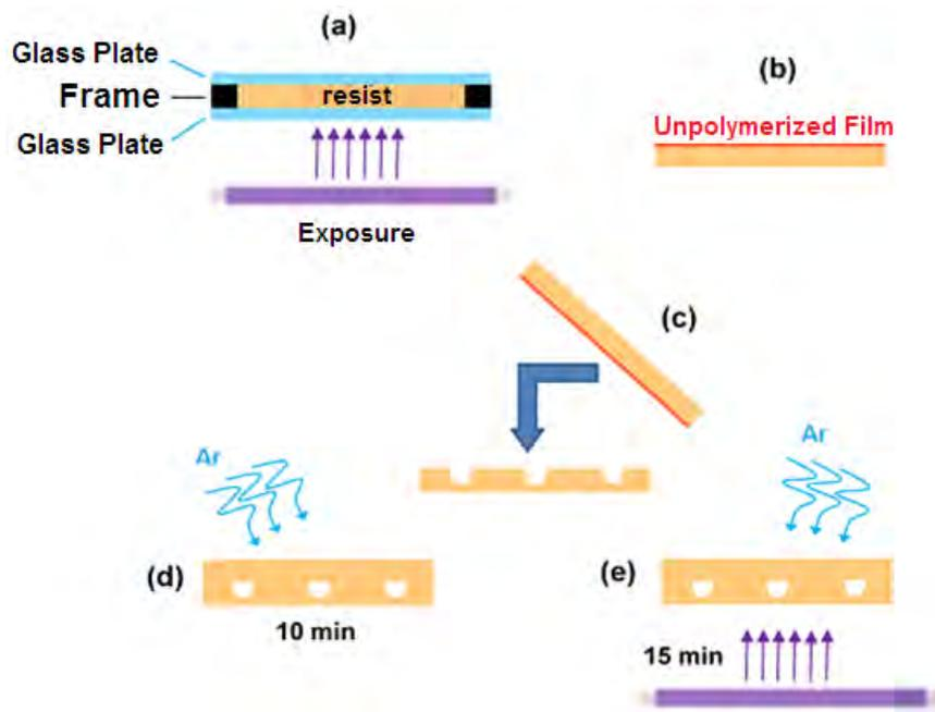
Figure 8 - Scheme of the fourth step: the sealing process. (Fonseca, 2008)
