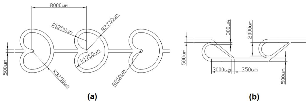
Figure 2 – Geometry of the pattern to be printed on the photomask with respective dimensions. (a) Omega geometry. (b) Tesla geometry.
