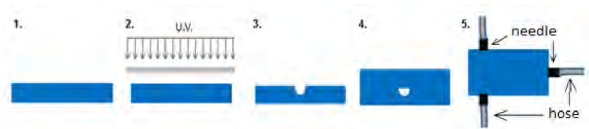
Figure 1 - Scheme of the photolithography micro-fabrication process
