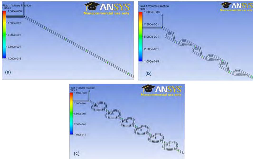
Figure 12 - Geometry of microchannels. (a) Straight. (b) Tesla-shaped. (c) Omega-shaped.
