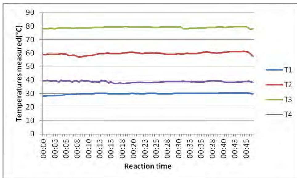
Figure 18- Temperatures measured in the respective thermocouples. T1: Room temperature. T2: Microreactor outlet temperature. T3: Aluminum plate temperature. T4: Soybean oil inlet.
