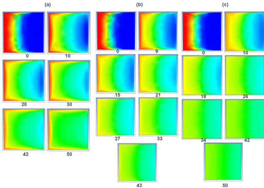
Figure 13 - Detail of the sections of the micromixers with the respective positions of the section (mm). (a) Straight; (b) Tesla; (c) Omega.
