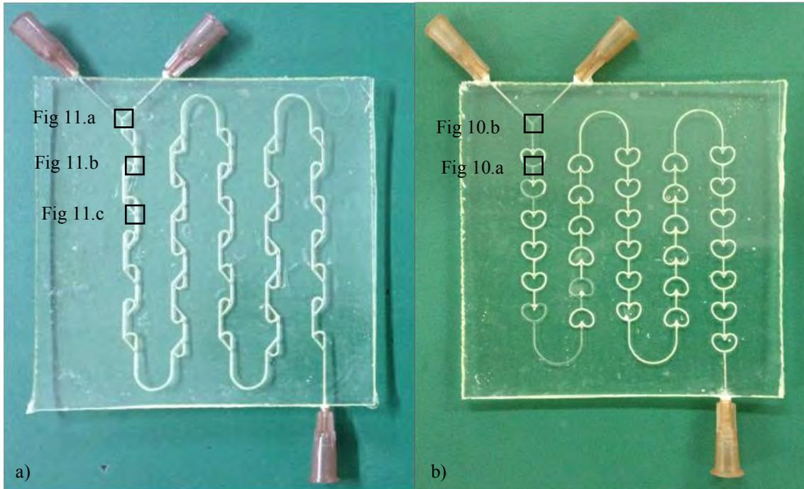
Figure 9 - Microreactors manufactured with the micro-channels communicated with the outside world through hypodermic needles. (a) Tesla geometry. (b) Omega geometry.
