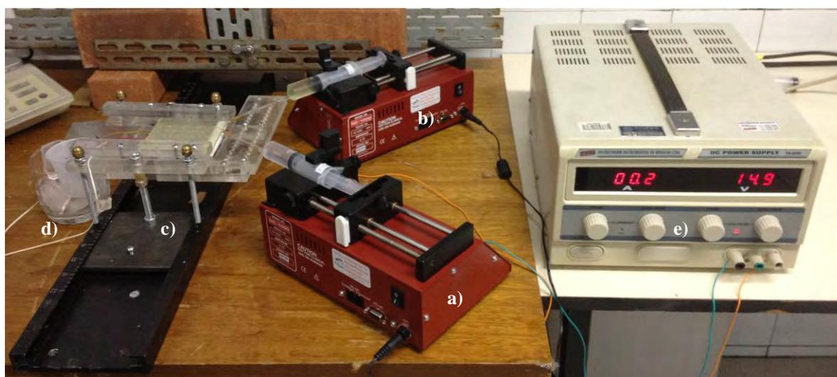
Figure 16 - Experimental setup. (a) syringe pump filled with solution of ethyl alcohol and NaOH. (b) syringe pump filled with soybean oil. (c) acrylic support with the microreactor fixed. (d) collection flask. (e) power supply.
