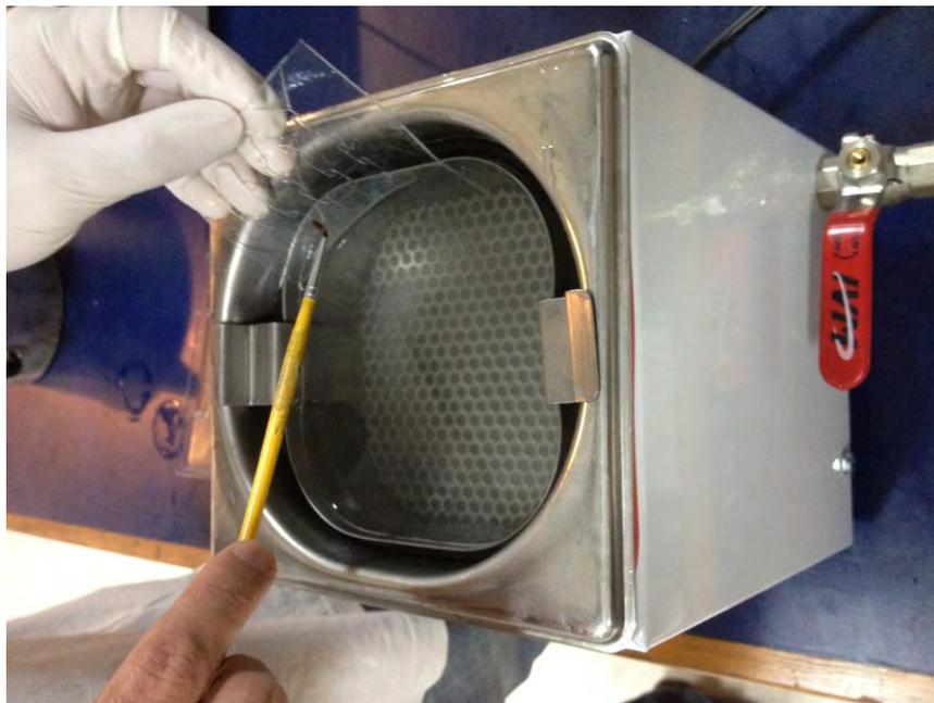
Figure 6 - Ultrasonic cleaner with the "develop" solution (water and detergent).
