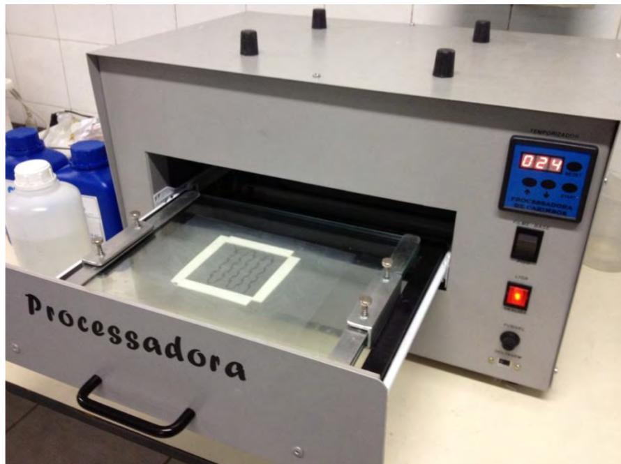
Figure 4 - Exposure of the photoresist by U.V. radiation
