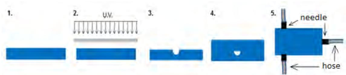
Figure 1 - Scheme of the photolithography micro-fabrication process
