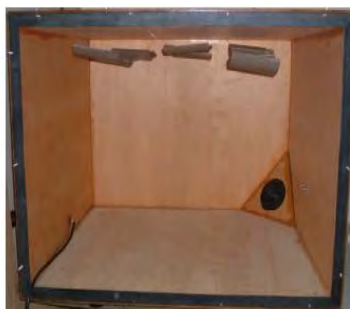
Figure 6. Reverberation chamber (receiving room).
