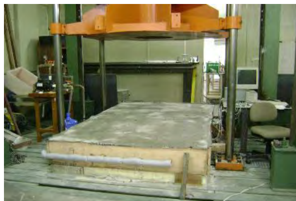
Figure 2 Appearance of the structure and the hydraulic machine used in the experiment.
