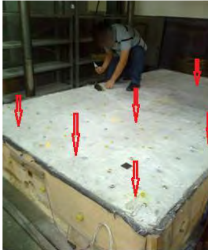
Figure 3. Placement of accelerometers on the plate. Marked in red excitation points.
