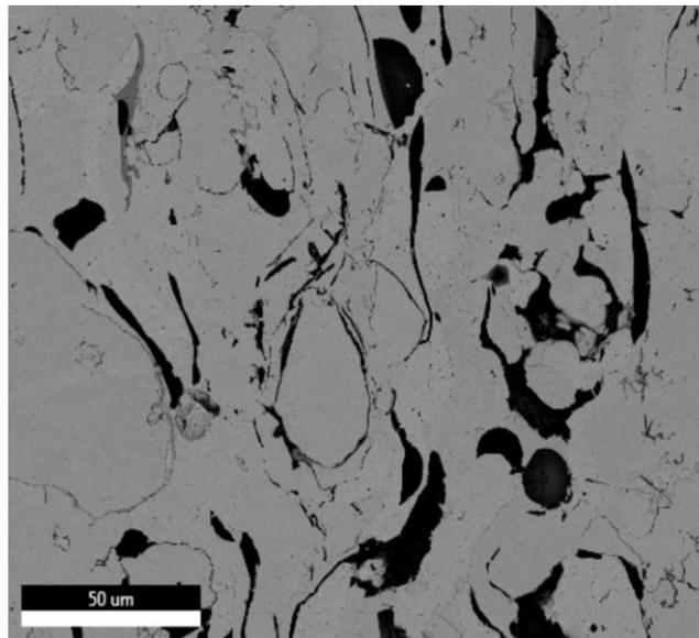
Figure 4. (a) Compositional image of the L<sub>1</sub> alloy layer.
