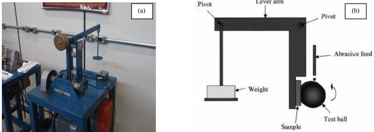
Figure 2. (a) Testing machine for micro-adhesive wear, Department of Materials Engineering - EESC-USP. (B) Illustration of the micro-adhesive wear equipment.
