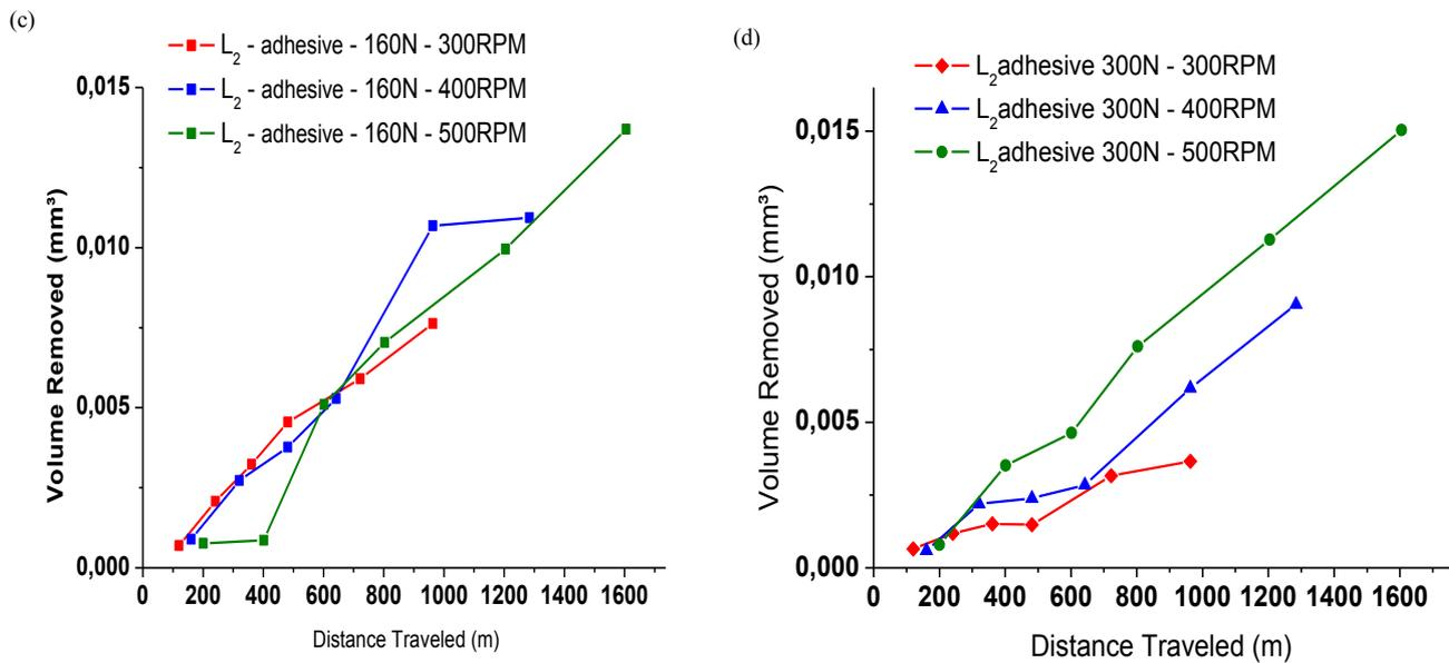
Figure 6. (a) Micro- adhesives wear tests: L<sub>1</sub> - 160N - 300, 400 and 500 RPM. (B) L<sub>1</sub> - 300N - 300, 400 and 500 RPM. (C) L<sub>2</sub> - 160N - 300, 400 and 500 RPM. (D) L<sub>2</sub> - 300N - 300, 400 and 500 RPM.
