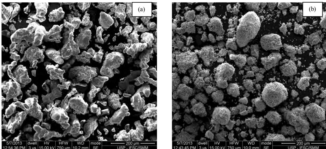
Figure 3. (A) Scanning electron micrograph of the powder alloy L<sub>1</sub>. (B) Scanning electron micrograph of the powder added for the production of alloy L<sub>2</sub>.
