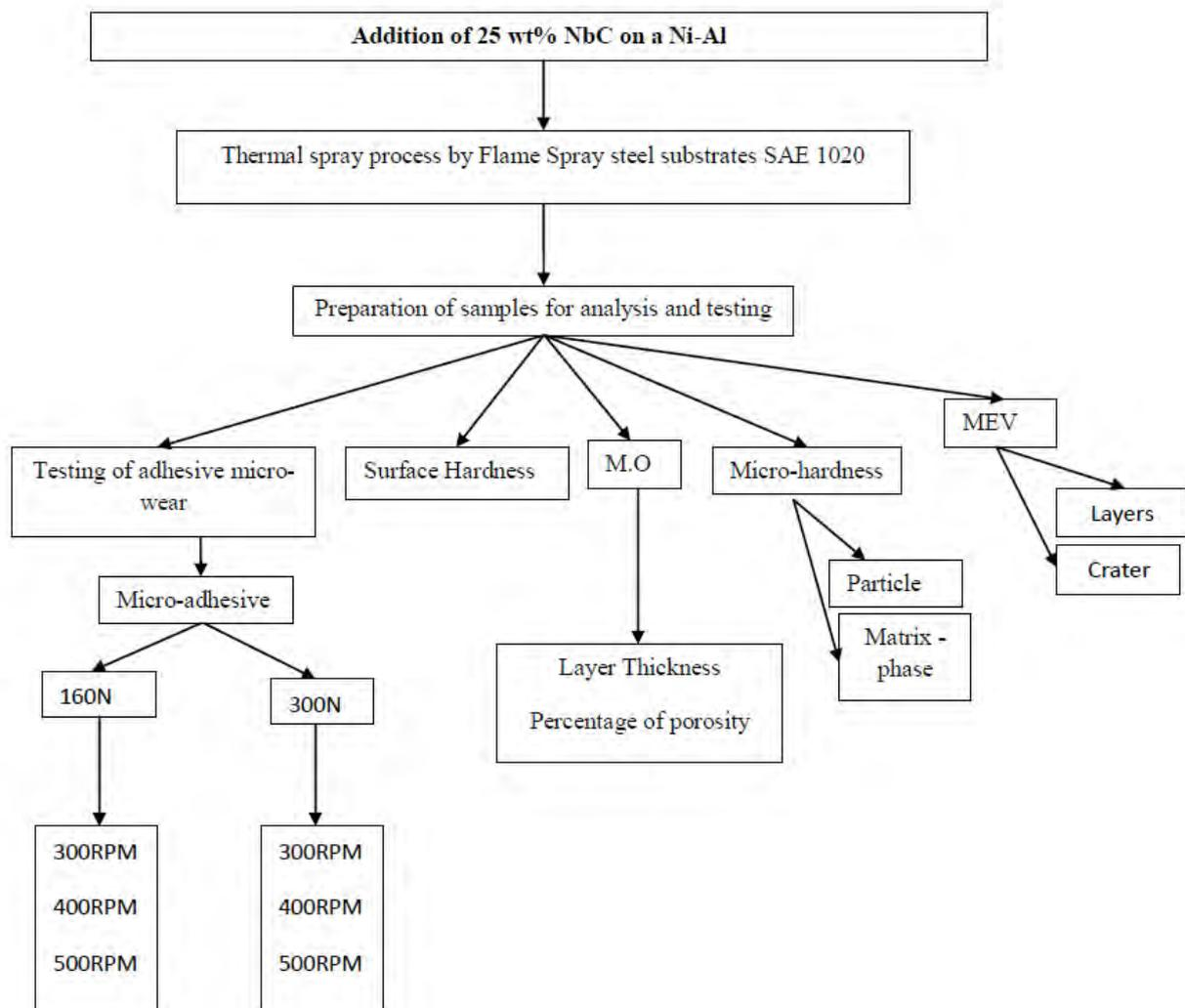
Figure 1. Flowchart of experimental work.
