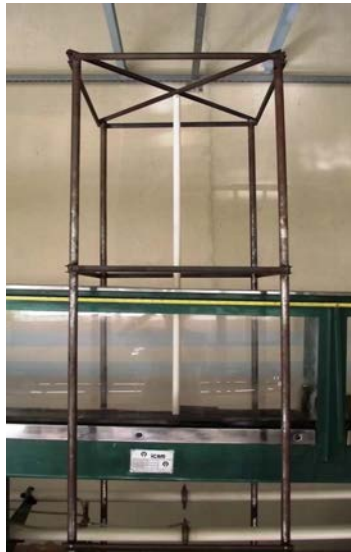
Figure 5 - Channel Currents and support for the cylinder
