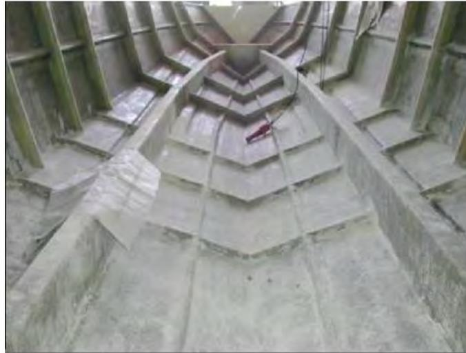
Figure 1. Structural arrangement of high speed boat built with composite material (Garcia, 2010).
