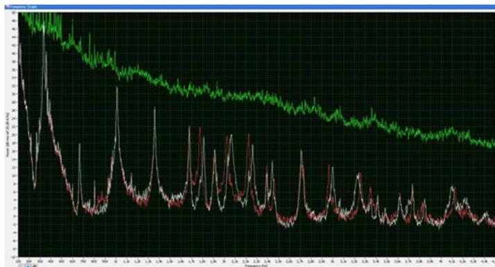
Figure 7. The difference of the isolation signal. The spectra in white and red are the inside microphones for measuring cell and the green is for the microphone outside the cell
