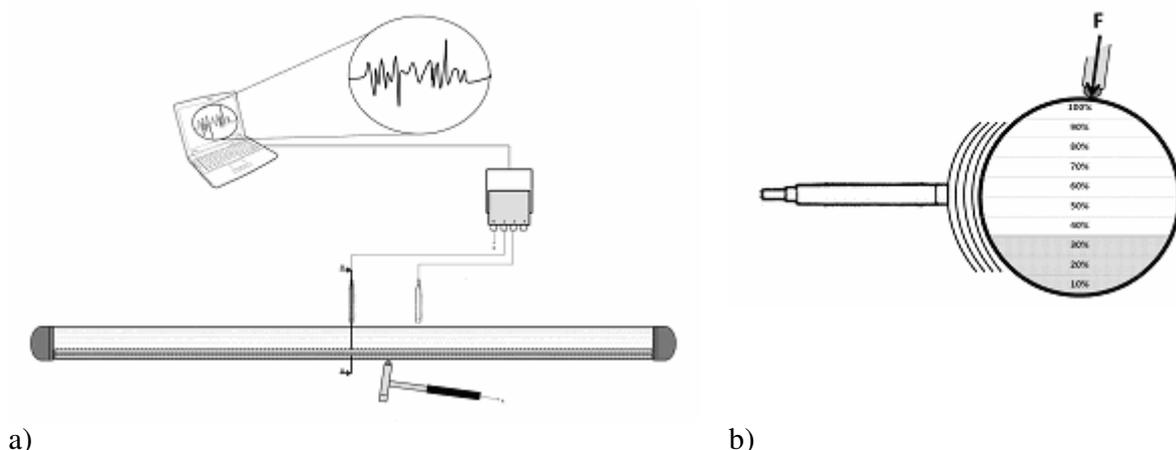
Figure 1. a) The scheme for determining patterns. b) The cut of the pipe test for better visualization of the phenomenon
