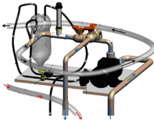
Figure 5. The experimental bench of two-phase flow
