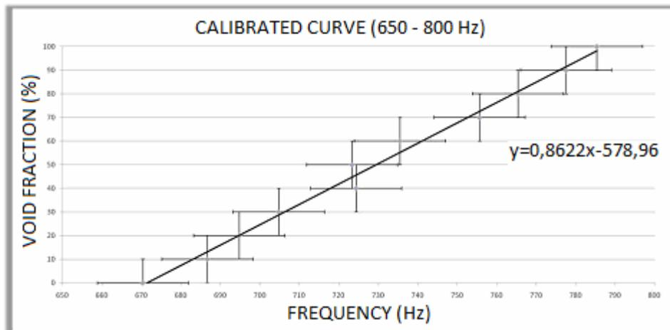
Figure 4. Curve calibrated to the range of 650 to 800 Hz, with a standard error and equation of a line
