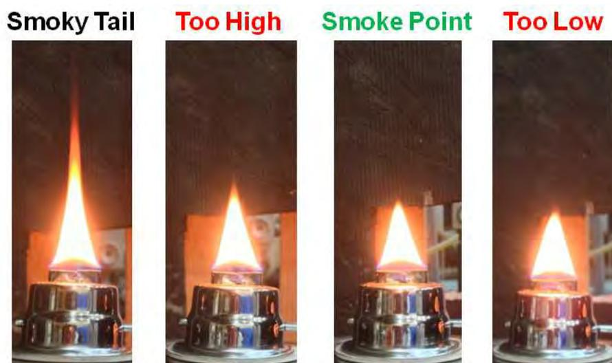
Figure 5. Different Stages of the Flame during the Smoke Point Determination
