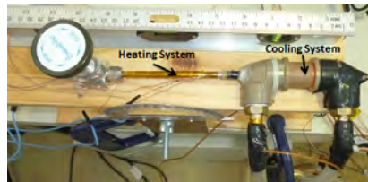
Figure 6. View of the heat pipe, showing the heating and the cooling systems.
