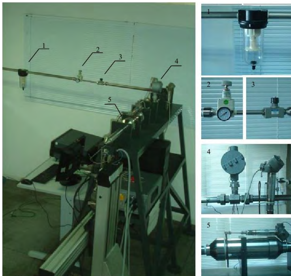
Figure 1 – Schematic of jet rig apparatus (1. Filter; 2. Pressure valve; 3. Precision flow control valve; 4. Flow meter; 5. Flow Straightener, Pressure and temperature probe).
