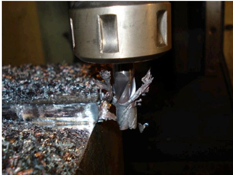
Figure 8 - Pasting at the end of life with TiAlN reground tool, v_c = 80\text{m/min} .
