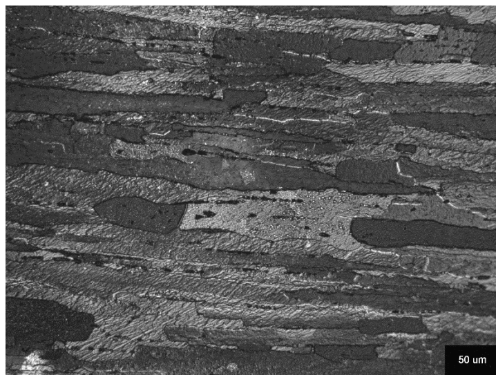
Figure 4. Microstructure from the T7451 specimen as received. Etching: Keller reagent.
