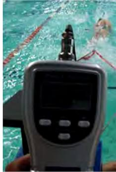
Fig. 3. The dynamometer used to measure tethered force of the swimmer.
