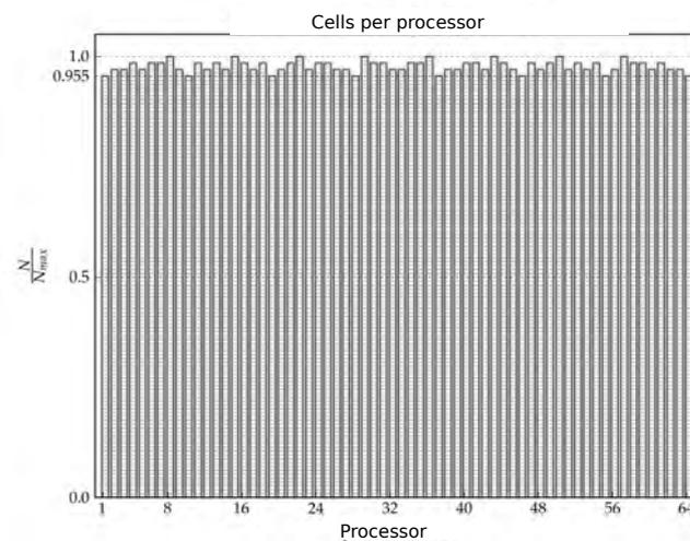
Figure 5: Load balance for the lid-driven cavity flow at  $Re = 400$ .
