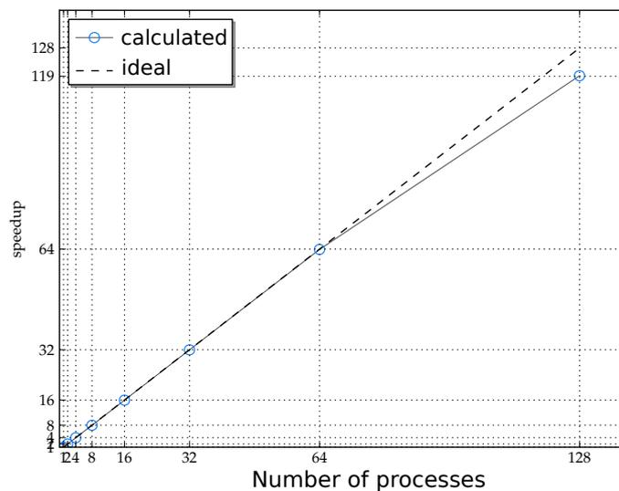
Figure 6: Speedup and ideal slope for the lid-driven cavity flow at  $Re = 1000$ .
