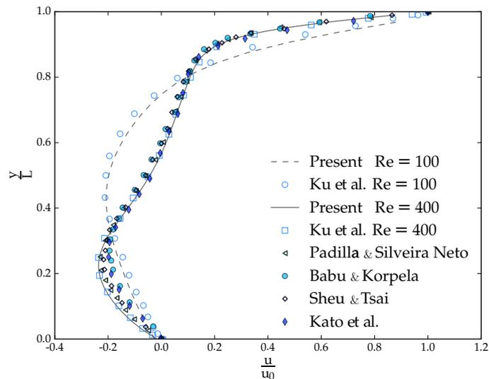
Figure 2: Velocity profile of  $u$  through the center of the cavity, passing by the point  $(x/L = 0.5; z/L = 0.5)$ . Comparisons are made to  $Re = 100$  and  $Re = 400$ .
