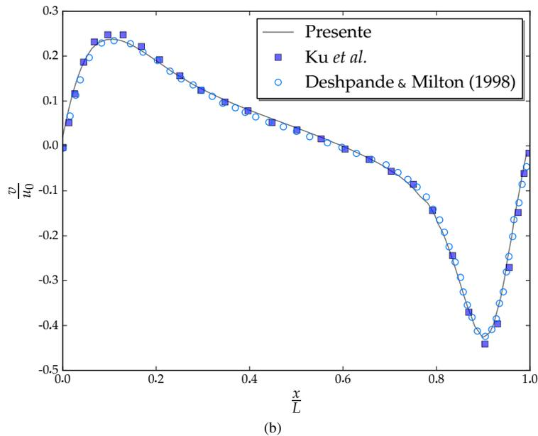
Figure 4: Velocity profiles in the lid-driven cavity flow. Comparison with the works of Ku *et al.* (1987); Deshpande and Milton (1998) with  $Re = 1000$ : (a) Component  $u$  over the vertical line  $y$  and passing trough the point  $(x/L = 0.5; z/L = 0.5)$  and; (b) Component  $v$  over the horizontal line in  $x$ , crossing the point  $(y/L = 0.5; z/L = 0.5)$ .
