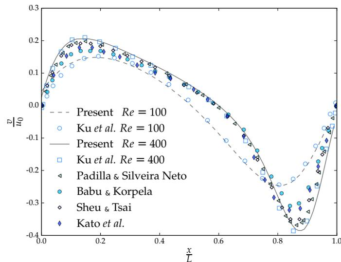
Figure 3: Velocity profile of  $v$  through the center of the cavity, passing by the point  $(y/L = 0.5; z/L = 0.5)$ . Comparisons are made to  $Re = 100$  and  $Re = 400$ .
