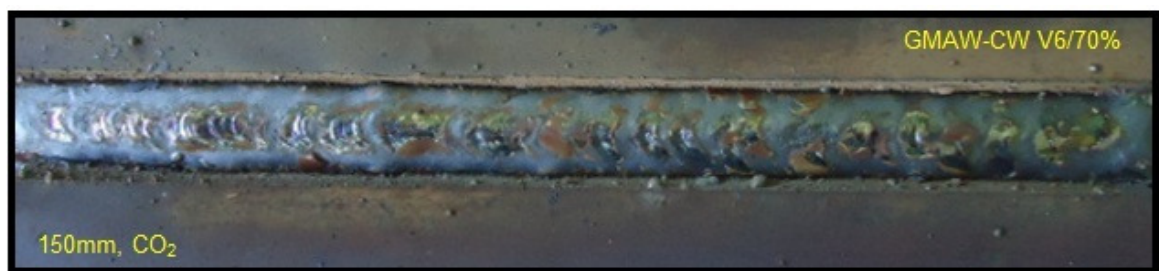
Figure 8 - Surface characteristics of the GMAW-CW process at set N6.
