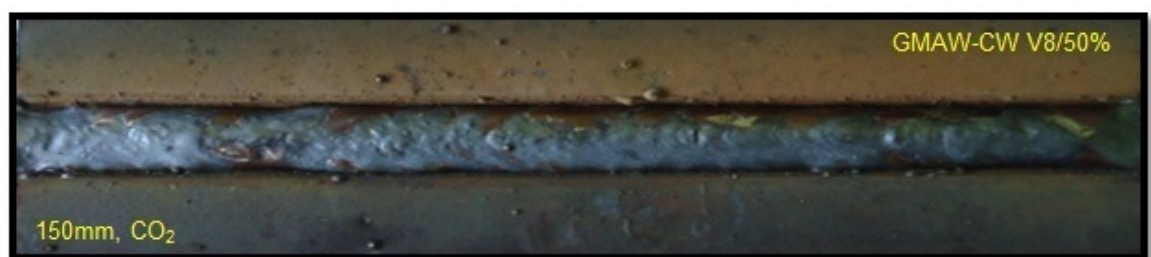
Figure 9 - Surface characteristics of the GMAW-CW process at set N7.
