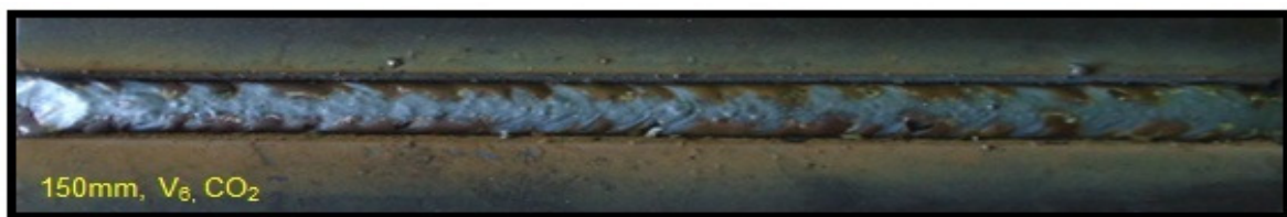
Figure 4 - Surface characteristics of the GMAW process at wire feed speed of 6 m/min.
