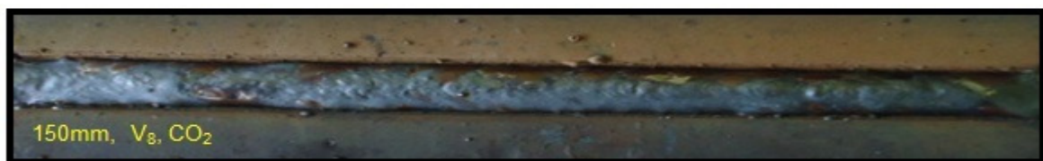
Figure 5 - Surface characteristics of the GMAW process at wire feed speed of 8 m/min.
