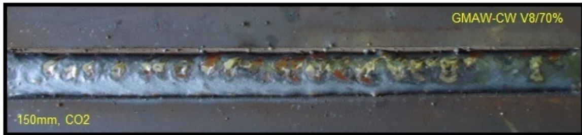
Figure 11 - Surface characteristics of the GMAW-CW process at set N9.
