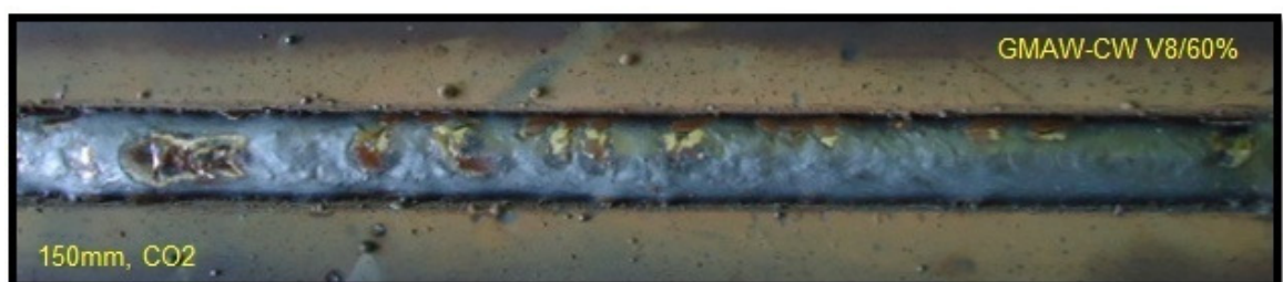
Figure 10 - Surface characteristics of the GMAW-CW process at set N8.
